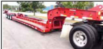
2014 FONTAINE 60 TON MODULAR, 26" DSR, 60" AXLE SPACING, 184" SWING CLEARANCE, SET UP FOR 2 AXLE JEEP, 14" DECK HEIGHT, AIR RIDE, ALUM WHEELS, 275/70R X 22.5 RUBBER, NON GROUND BEARING. IN STOCK. CALL FOR MORE INFORMATION.
