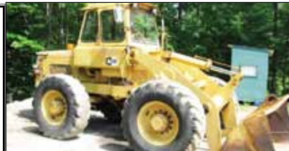
1965 Hough 50 2-yard Bucket Loader. Strong-running Int'l diesel, rear steer. Everything works. Includes 2 spare tires & rims, $7300 OBO. Mickey, 603-582-1005
