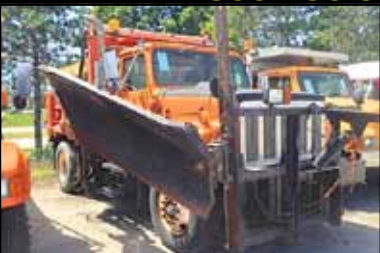
1996 IH 2554 10' GALLION DUMP, 10' PLOW & WING PLOW, DT466 230HP DIESEL, AUTO OD, SPRING, COVER, SS SANDER, 35K GVW, 164K MILES, STK#10743
