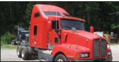
1996 Kenworth T600, 1,021,486 Miles, Cummins N14 Power, 12 F/A, 38 R/A on Air, Single Frame...$12,500 Call Bill 781-439-6000
