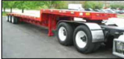
2014 DORSEY 50 TON STEP DECK, 3 AXLE, LIFT IN MIDDLE, HD 8" SIDE RAIL, 6" CROSSMEMBERS, 12" ON CENTER, LED LIGHTS, 255 LO PRO TIRES, CALL FOR MORE INFORMATION.
