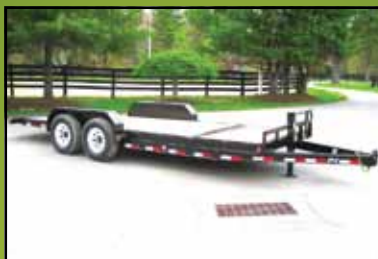
2013 PJ T6 20ft split tilt 16 tilt portion, 14,000lb GVWR, Torsion Suspension $5,995
