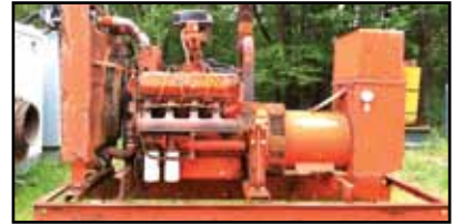
PINCOR 85KW GENERATOR. 277/480 Three Phase, International Engine, Natural Gas, 1120 Hours
