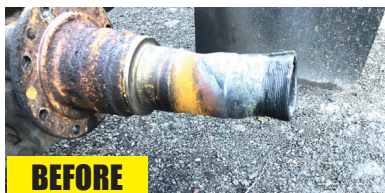
TRUCK DRIVE SPINDLE REPLACEMENT WELDED IN PLACE
