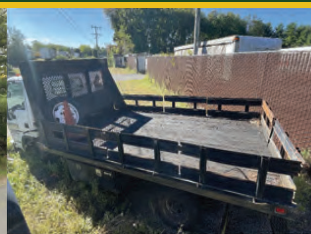
14FT RACK BODY $3000 34" Frame width, wooden floor, removable side panels, drivers side tool box, multiple available.
