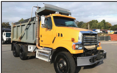
2009 STERLING T/A DUMP. MBE - 410 Hp, 8LL, 20k Front, 46k Rears., Spring Susp., 14ft Steel Dump Body, Clean, DOT Ready. 108,946 Miles. #AH8468, $51,500
