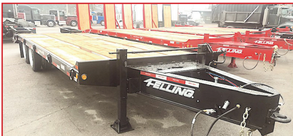
2026 FELLING FT 40. 22' deck, 6' Double incline Beavertail, 30" Spring Assisted Ramps, 16 D Rings, Oak Decking, A Frame Tool Box, Black Paint
