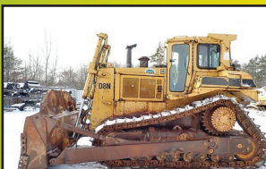
1988 CATERPILLAR D8N: 17,302 Hours, 13 Ft Semi-U Blade, Cab W/ A/C, Good U/C, Diff Steer, 6 Cyl Cat 3406 Turbo, 1 Owner, 85K Lbs, stk#DZ536, $64,500
