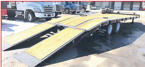
2026 FELLING FT 45. 22' deck, 6' Double incline Beavertail, 38" Air Assisted Ramps, 16 D Rings, Oak Decking, A Frame Tool Box, Black Paint
