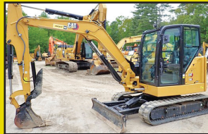
2020 CATERPILLAR 306CR: 438 Hours, 12" Digging Bucket, Hydraulic Thumb, 78" Angle Blade, Cab W/ A/C, Swing Boom, 4 Cyl Cat Turbo, 57 HP, 16k Lbs, stk#XC531B, $79,500
