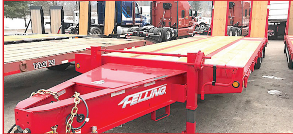
2026 FELLING FT 45. 24' deck, 6' Double incline Beavertail, 30" Air Assisted Ramps, 16 D Rings, Oak Decking, A Frame Tool Box, Red Paint
