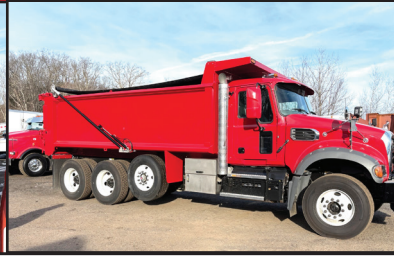
Custom Severe Duty Dump Bodies With 1/4" Hardox Sides And 3/8" Hardox Floors
