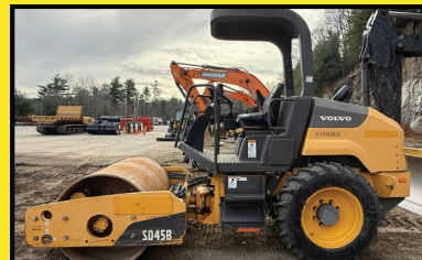
2017 VOLVO SD45 OROPS, 54" SMOOTH DRUM, VIBE DRUM, DRUM DRV, 438 HRS $42,500
