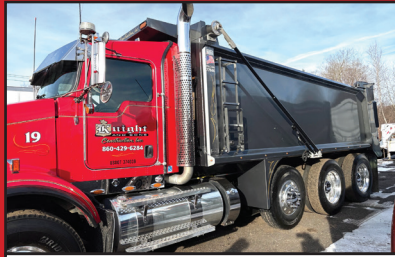
Custom Severe Duty Dump Bodies With 1/4" Hardox Sides And 3/8" Hardox Floors
