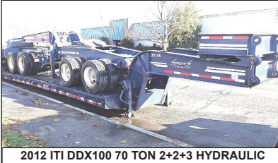
2012 ITI DDX100 70 TON 2+2+3 HYDRAULIC EXTENDABLE STEERABLE TRAILER. Air Ride. Comes With 10' Flip Up Gooseneck Ext, Self-Contained Power Unit, 30' Deck, 8' 6" Wide, JP40 Tandem Axle Jeep, B80 Tandem Axle Stinger With Pin On 3rd Axle. Wireless Remote, Super Singles. Call For More Information.
