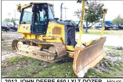
2012 JOHN DEERE 650J XLT DOZER , Hours 12K, 8' 6" Blade, Trimble Onsite GPS System, One Owner, Fleet Maintained, Original Paint, Recent Bottom (Tracks), Full Cab, Heat, A/C, Loaded. Call For More Information.
