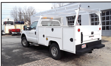
DURA MAG SERVICE BODY. All Aluminum, Heavy Duty Ladder Rack
