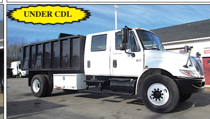
2007 INTERNATIONAL 4300: DT466-260HP, PRE-EMISSIONS, 87K MILES, ALLISON 3500RDS AUTO, 26K GVW, SPRING SUSP, 5.64 GEARED RATIO, 11R 22.5 TIRES, SINGLE FRAME, AIR-BRAKES, A/C, PTO NEW 14' STEEL DUMP, BARN DOORS, PINTLE, AIR-TO-REAR, TOOL BOX. $45,000
