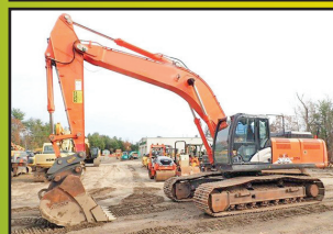
2016 HITACHI ZX350LC-6N: 8,337 Hours, 66" Bucket, Hydraulic Coupler, A/C, 6 Cyl Isuzu Turbo, 281 HP, 78K Lbs, stk#XC160, $79,500
