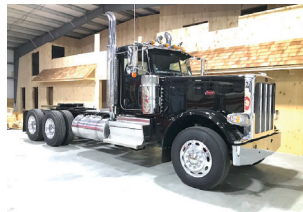
2020 PETERBILT 389 EXT HOOD. 565 Cummins, 18 Speed, 46k Rears, Front Disc Brakes, Platinum Interior, 128k Miles, Wet Line, 10k Ext Warranty, $185,000.
