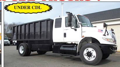
2009 INTERNATIONAL 4300: DT466-260HP, 155K MILES, ALLISON 3500RDS AUTO, 26K GVW, SPRING SUSP, 5.64 GEARED RATIO, 11R 22.5 TIRES, SINGLE FRAME, AIR-BRAKES, A/C, PTO, NEW 15' STEEL DUMP W/ BARN DOORS, PINTLE PLATE, AIR-TO-REAR, TOOL BOX. $40,000
