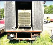
GENERATOR. Self Contain In Trailer, Cummins 855, Model 440FDR71112JJW, 250 KVA, 200 KW, 480 Volt, 300 AMP, 275 Gallon Fuel Tank, \$7,500.
