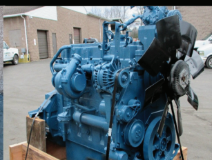
INTERNATIONAL DT466P - $3500 Pre-tested International DT466P Mechanical, 175HP @ 2300RPM. Set up for hydraulic brake application.
