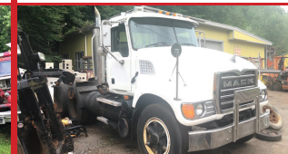
2005 MACK GRANITE TRACTOR. E7 Mack Motor, 10 Speed, 2 Line Wet Line, 48K Rears, 14K Fronts, $35,000
