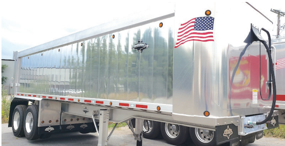
2023 TRAILSTAR 28X96 ALL ALUMINUM SMOOTH SIDE DUMP TRAILER. Air Ride With Front Lift Axle , Aluminum Wheels ,Mandoor , 2-Way Gate , 60 Inch Sides , Extra Lights . Owner Operator Spec's
