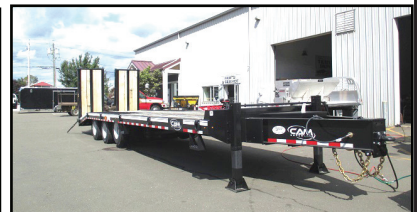
CAM SUPERLINE 65K DECKOVER TRAILER. 8' 6" x 32', 5' Beavertail, 40" x 142" Bifold Air Powered Ramps, Air Lift Axle, #525645
