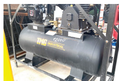
NEW TMG Industrial 40 Gallon 2 Stage Air Compressor. 4 Stroke OHV, 175 PSI, 302cc Engine, $2,000
