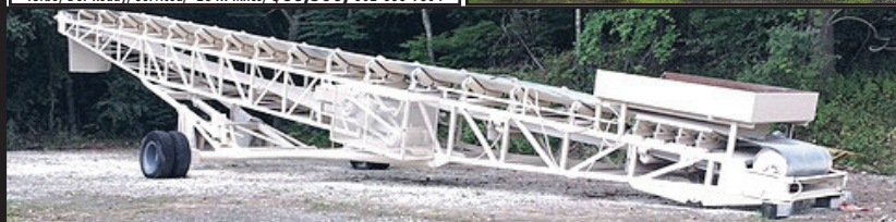
BARBER GREEN 42" X 60' RADIAL STACKING LATTICE CONVEYOR. 30 HP, 240/480 Volt, 3 Phase Motor, Wrap Drive, 54" Wide X 42" Deep Truss, 3.5" X 3.5" X 3/8" Angle Truss, Very Rugged Conveyor, Conveyor Belt In Good Condition, No Major Tears, $28,000 . Gales Ferry, CT 860-460-0767
