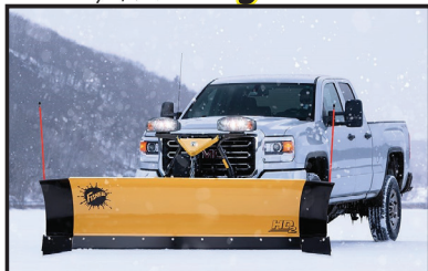
HD2™ - Straight Blade available in 7' 6", 8', 8' 6" and 9' widths
