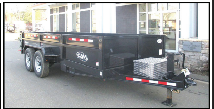
CAM SUPERLINE 15.4K LOW PROFILE HEAVY DUTY DUMP TRAILER. Tubular Mainframe, Slipper Spring Suspension, #530174
