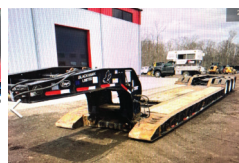
2011 ETNYRE BLACK HAWK. 55 Ton Non Ground Bearing. 26' Well. Air Ride. With Rear Lift, $45,000
