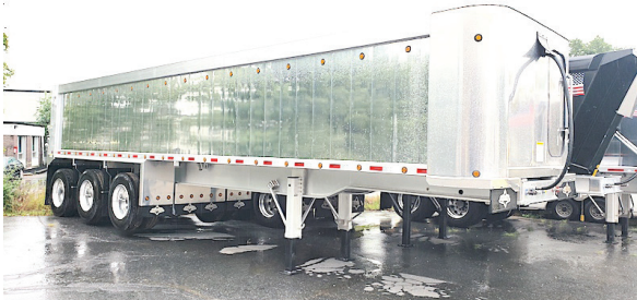
2023 TRAILSTAR 36X96 ALL ALUMINUM SMOOTH SIDE DUMP TRAILER. Air Ride (Front And Middle Axle Lifts ) All Aluminum Wheels, 60-Inch Sides, Mandoor, 2 Way Tailgate , Extra Lights On Sides And Rear . Loaded Up Owner Operator Specs
