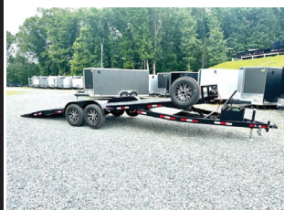
BCL 82 x 24 Full Power Tilt, Steel Deck With 12K Winch 14,000Lb. GVWR, $10,900
