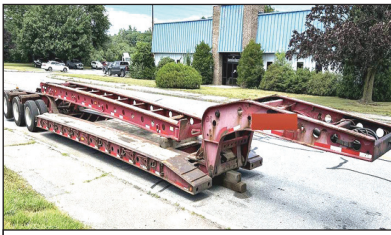
1998 FONTAINE, MODEL. 50 Ton, Detaches At Both Ends, 25' Flat Level Deck - 20" Loaded Deck Height, 25' Beam Deck Insert, 20" Loaded Deck Height, Non Ground Bearing, Air Ride, Boom Trough & Deck Cut Out, Lift Axle, Outriggers, Aluminum Wheels, Strobe Lights. Call For More Information.
