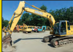
2006 JOHN DEERE 160C LC: 6,274 Hours, 48" Bucket, Hyd Coupler, 2 Speed, A/C, Good U/C, 4 Cyl John Deere Turbo, 36K Lb Size Class, STK#XC100, $53,500
