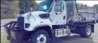
2017 FREIGHTLINER 114SD PLOW TRUCK. Detroit DD13, 370 HP, 10' Monroe 5-7 Yard Body, Monroe Snow Plow, Power Cover, PS, PW, PL, #JB2422
