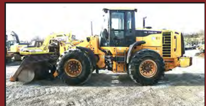
2015 HYUNDAI HL740TM-9A. Heat-A/C, Cummins Power, Aux. Hydraulics, JRB Coupler 3.5 Yd. Bucket, Forks, 20.5 Rubber, Backup Camera, 4160 Hrs, Coming In
