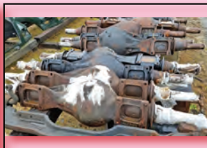
REAR AXLE HOUSINGS. CAST, STEEL, AIR RIDE AND CAMELBACK.
