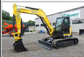
2017 YANMAR SV100-2: BRAND NEW, FULL ENCLOSED CAB, QUICK COUPLER, HYD. THUMB, 36" DIGGING BKT. & BLADE, A/C. CALL FOR MORE INFO & PRICING.
