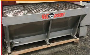
Sno Bandit salt & sand spreader. Elec drive, stainless steel. 1.7 cu yards, pintle chain feed. $4500.
