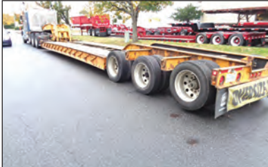
2006 ROGERS 50 TON LOWBOY TRAILER, Tri Axle, Air Ride, Air Lift 3rd Axle, Detachable Neck, 27' 8" Deck, 102" Wide, Call For More Information.
