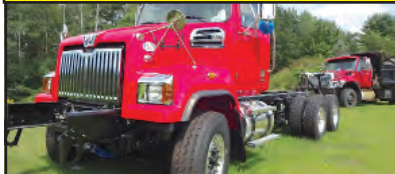
2018 WESTERN STAR 4700SF CAB & CHASSIS. Detroit DD13, 505 HP, Allison Auto, 46K Rear, 20K Front, Aluminum Wheels, #JT6293
