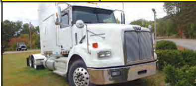
2013 WESTERN STAR 4900SA TRACTOR. Detroit Power, Eaton Fuller 10 Speed, Air Ride, 40K Rear, 13K Front, #FK2999, $54,999
