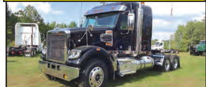
2018 FREIGHTLINER 122SD TRACTOR. Detroit DD16, 600 HP, Eaton Fuller 18 Speed, Mid Roof Sleeper, Air Brakes, Aluminum Wheels, #JT1907
