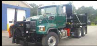
2016 Western Star 4700 SF Everest 14' side dump, Everest power tilt front plow hitch, front plow control, Everest hydraulic patrol wing system, Detroit DD 13, 470 HP, #WHH0663
