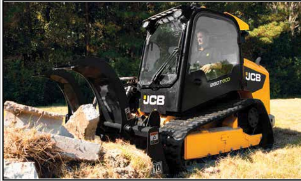
2016 JCB 260T. 74 HP, Heat/AC Cab, Air Susp Seat, Radio, Block Heater, 2 speed, Smooth Ride, ISO & Dual Pattern Controls, Creep Speed, 7 Function Joystick.
