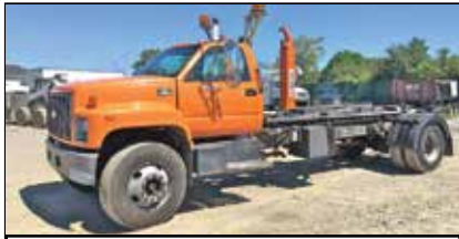
2001 GMC 7500 SWAPLOADER. 22,000 lb Hook Lift, 33,000 GVW, Propane Fuel Engine, Automatic, 77,000 Miles, Exceptionally Clean, $35,000. OBO 978-465-7757
