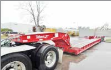
1999 TALBERT 51 TON TRAILER, NON GROUND BEARING, AIR RIDE, TRI AXLE, 24' DECK, 22' DECK HEIGHT, LIFT ON THIRD, 255/70/22.5 TIRES MOUNTED ON ALUMINUM HUB PILOTED WHEELS, OUTRIGGERS, D-RINGS, COMPLETELY RECONDITIONED, SANDBLASTED & PAINTED, NEW BRAKES, SEALS, DECKING, HUBCAPS, FLAPS, DECALS, DOT TAPE. ONE OWNER. CALL FOR MORE INFORMATION.
