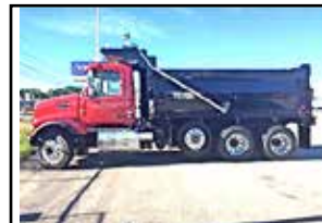
2017 VOLVO VHD84F200. 17' Beaurac Diamond-DH Body, 475HP, I-shift, 20k FA, 46K RA, 3.73 Ratio, 20k Steerable Pusher Axle, T-Ride Susp, PH Mirrors.
