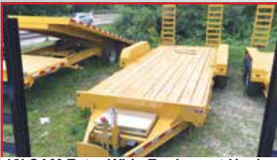
18' CAM Extra Wide Equipment Hauler. model 7CAM18CXW, 83" usable deck width, pallet fork carrier, 8 stake pockets, 6 D rings, 7K jack, aluminum tool box, 16,100 GVW, $5,995
