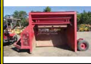
1987 READ RD402: 2,253 HOURS, 3 YARD, 2 1/4" TOP SCREEN, 1/2" SLOTTED BOTTOM, 3 CYL LISTER DIESEL, 9'10" OPENING, GOOD RUBBER, STK#SC387, $28,500
