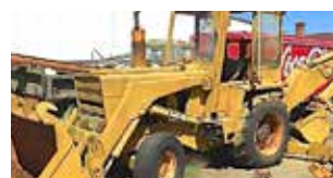
Unihoe Backhoe Loader w/ 2 yd bucket, 1 yd hoe bucket, digs over 15' deep, 3 cyl Detroit Diesel, Runs Great, $7,500/ BO
