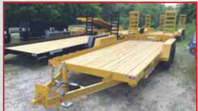
18' Equipment Trailer model 4EC18, 8 stake pockets, 7K jack, 102" wide, 9996 lb GVW, $3,995
