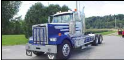
2017 Western Star 4900EX. Detroit DD16, 600 HP, Eaton-Fuller 18 speed, Airliner suspension, chrome bumper & exhaust, #JC7829
