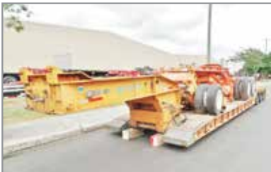
1994 ROGERS 60 TON 2+2+2, AIR RIDE, 102" WIDE, NON GROUND BEARING, LO PRO HUB PILOTED TIRES AND WHEELS, 24' DECK, CAN BE RUN AS 2.3 OR 4, OR AS A 2+2+2. COMES WITH 2 AXLE JEEP, GOOSE NECK EXT, 2 AXLE TRAILER, 2 MORE ADDITIONAL AXLES AND ROGERS SPREADER BAR. VERY LOW MILES, ORIGINALLY BUILT FOR MOHAWK POWER IN NY. D-RINGS AND OUTRIGGERS. CALL FOR MORE INFORMATION.
