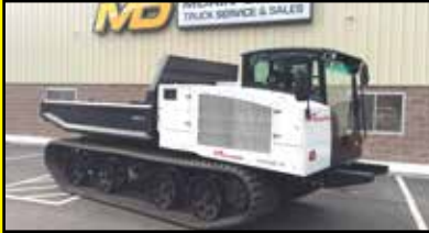
2017 Prinoth Panther crawler carrier, versatile utility vehicles. Just about any implement can be fitted to the PANTHER's 860 mm (34 in.) truck-inspired chassis with little to no modifications, making installation simple and easy.
