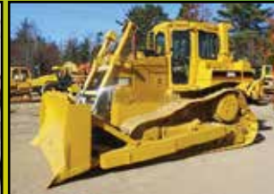
1996 CATERPILLAR D6H XL-II: 12,242 HOURS, 6-WAY, CAB W/ A/C, HIGH TRACK, 6 CYL CATERPILLAR 3306 TURBO, 42K LB SIZE CLASS, STK#DZ440, $39,500
