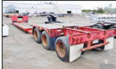
1997 TRAIL KING DOUBLE DROP DECK EXTENDABLE TRAILER, TRI AXLE, PIN ON THIRD, AIR RIDE, DETACH NECK, 98" WIDE, 22.5 RUBBER, LOCATED IN COLUMBUS OH. CALL FOR MORE INFORMATION.
