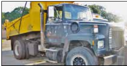
1995 FORD L8000 DUMP. 8.3 Cummins, 5 spd., A/B, 33K GVW central hydraulics, plow frame, sander controls 10' 8 yd. body W /chutes, pintle w/air to rear, runs well, 800-464-0573, www.WestsideTruckEquipment.com
