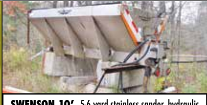
SWENSON 10' , 5-6 yard stainless sander, hydraulic driven from truck, fits 26K GVW & down vehicles, will need track from sitting, other units & 10-11' PA plows available, 800-464-0573, www.WestsideTruckEquipment.com
