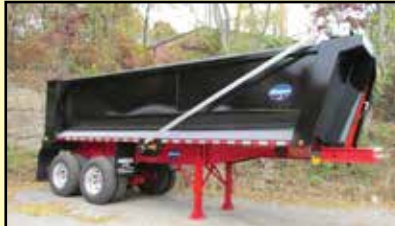
2016 26' RHODES STEEL DUMP, 70,000#, SINGLE POINT, HIGH-LIFT GATE.
