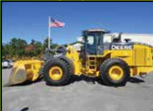
2013 JOHN DEERE 744K: 1,355 HOURS, 5.25 YARD, CAB W/ A/C, 6 CYL JOHN DEERE TURBO, RIDE CONTROL, AUTOSHIFT, TRACTION CONTROL, GOOD RUBBER, 56K LB SIZE CLASS, STK#L0303, $237,500
