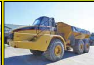
2005 CATERPILLAR 740: 11,510 HOURS, 40 TON, 6X6, ARTIC., CAB W/ A/C, 6 CYL CAT 3406 TURBO, STK#HT148, $87,500
