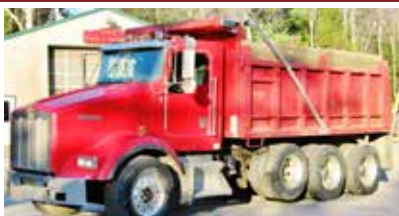
1997 KW T-800. CAT 3406E @ 475 H.P., 10 spd, 20F + 20L + 46R on rebushed Hendrickson w/ new springs, perfect dbl frame, 16 foot steel body, 514K miles, $50,000.
