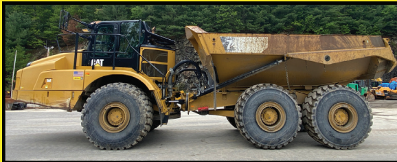
2020 CAT 740GC A/C, 3RD VLV HYD, 55 HYD Q/C, 1.5CY GP BKT, 74HP TIER-4 DSL, HI-SPD TRVL, RIDE CTRL, 405/70R18 TIRES, 7,448 HRS $219,000
