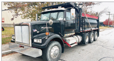
2017 WESTERN STAR TRI AXLE DUMP TRUCK. Glider Kit, No Emissions, Model: 4900, Original 320,000, 17' Body, 60 Series Detroit 500 Hp, 8 Speed 8 LL, 46 Rears Full Lockers, 20K Pusher Axle, 18K Front, Electric Canvas, Air Gate, Perfect Double Frame, One Owner, Fleet Maintained. Call For More Information.
