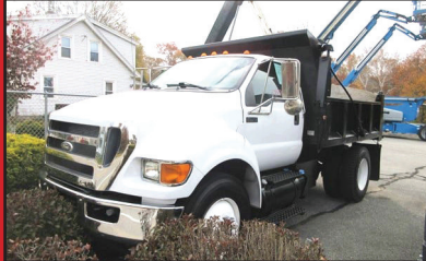
2012 FORD F750XL DUMP TRUCK , Cummins ISB 6.7L Diesel, Allison Automatic Transmission, Ledwell 10' Long x 2' High Steel Body, Manual Roll Tarp, Double Tailgate Chutes, Chelsea PTO. $31,900
