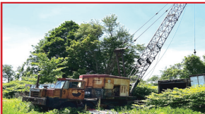
LORAIN CRANE. 40 Ton, Cummins Lower Motor, Detroit Upper Motor, 12' Boom
