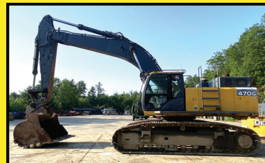
2016 DEERE 470GLC A/C, 11' STK, HYD Q/C, 72" BKT, 367HP TIER-4 DSL, 36" TG PADS, 7,899 HRS $129,000
