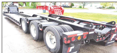
2023 FONTAINE WORKHORSE 55LCC FLD. Tri Axle, Air Ride, Set Up For 4th, Air Lift On Third, 18' Deck Height, 26' Deck, Dual Cam Pawl Assembly With 7 Ride Height Positions, Removable Kingpin At 108 Inch Radius, Alternate Kingpin At 96" Radius, 275 Rubber, Alum Wheels, Not Spreader Bar Or Goose Neck Extension Capable, Just Off Short Term Lease, Call For More Information.
