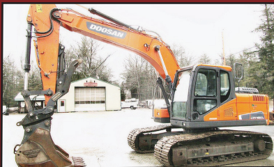
2017 DOOSAN DX180LC-5. 3647 Hrs, 36" Bucket, Coupler, Full Rotation Thumb, 44,000 Lbs., $99,000.
