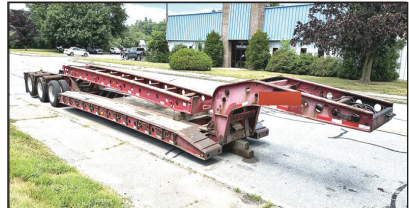
1998 FONTAINE, MODEL. 50 Ton, Detaches At Both Ends, 25' Flat Level Deck - 20" Loaded Deck Height, 25' Beam Deck Insert, 20" Loaded Deck Height, Non Ground Bearing, Air Ride, Boom Trough & Deck Cut Out, Lift Axle, Outriggers, Aluminum Wheels, Strobe Lights. Call For More Information.
