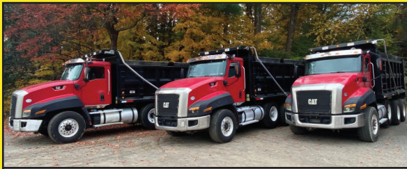
(3) 2015 CAT CT660 TRI-AXLE DUMP TRUCKS CAT CT13 430HP DSL, EF 8-SPD MNL TRANS, 62K LB GVWR, AIR LIFT PSHR AXLE, HENDRICKSON RTE SPRING SUSP, 204" WB, DBL FRM, OX BODIES 16'L x 4'6"H STL BDY, 135K+ MI $99,000 EACH
