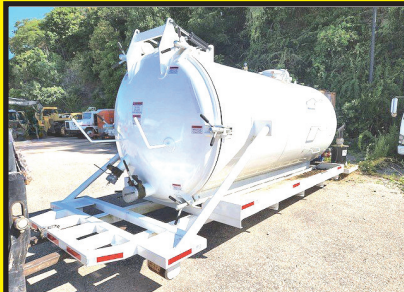
ROLL-OFF LIQUID VACUUM TANK. 3500 GAL, ROLL-OFF FRAME APPLICATION, RCF 870 FRUITLAND VAC PUMP, 512 CFM HYD DRIVEN FROM WET KIT ON TRUCK, HYD. HOSES, QUICK DISCONNECTS, $60,000 OBO. 401-255-3100
