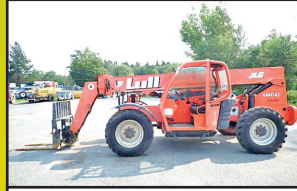
2010 LULL 644E-42: 6,784 Hours, 6k Lb Lift, 42 Ft Lift Height, 4x4, Orops, 4 Cyl Cummins Turbo, Tilt Body, Traversing Carriage, stk#FL806, $33,500
