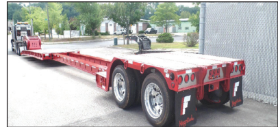
IN STOCK - 2023 FONTAINE LXTN40. 40 Ton Extendable, 34' Closed - 60' Open. Also Available 29' Closed - 50' Open. Tandem Axle, Set Up For 3rd, Air Ride, Non Ground Bearing, 102" Swing Clearance, 20" Deck Height, Alum Wheels. In Stock, No Waiting. Available In Manchester NH And At The Factory In Springfield AL. 3rd And 4th Axles Available. Call For More Information.
