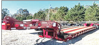
NEW MODEL - IN STOCK - 2023 FONTAINE MAGNITUDE 60HD-MX. Deck Extends From 30' To 51', 65 Ton When Closed, Built To Handle A 60 Ton Load With Ease, 30' Clear Deck Length Extends To 51', 22" Loaded Deck Height, 6" Ground Clearance, 7 Position Hydraulic Detachable Gooseneck, 7 Position Air Ride Tridem Bogie, 402 Jeep Ready, 36" And 83" Flip Box Ready, 60/90 Flip Axle Ready, EQ2 Spreader Bar Ready, Loaded. Call For More Information.
