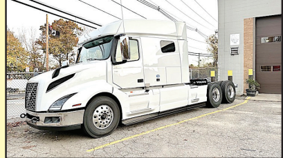
2024 VOLVO VNL64T740, D13-455HP, 12SPD. I-SHIFT, 13,200# FRONT / 40,000# REARS, AIR-RIDE SUSPENSION. #230133
