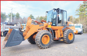
2011 CASE 621E. 2 3/4 Yd. Bucket, ACS Quick coupler, 3rd Valve Hyd., A/C, Heat, 5,351 Hours. # 3124, $57,000.
