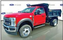
2024 FORD F-550 SD XL DRW W/9' UNICELL ARIFLOW 4-5 YARD DUMP 4WD. 6.7L Diesel, Auto, AC, PW, PL, Snowplow Prep, 19,500 GVW, \$78.190.
