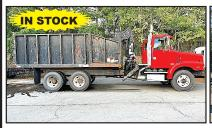
2000 VOLVO WG64B, 275HP., AUTO, 16,000# FRONT / 40,000# REARS, JOHNSERED 820 CORTU CRANE, 20' DUMP BODY. #210299A
