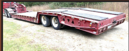
2006 TRAIL KING 35 TON DETACHABLE LOWBED. HYDRAULIC TAIL, WINCH, 8'6" WIDE, 21' DECK, 8' OVER WHEELS, AND 8' TAIL, $34,500. 603-759-5918
