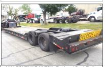
2001 FONTAINE 35 TON. Flat Level Deck Trailer With Beaver Tail. 24' Deck, 4' Beaver Tail, Power Pack, Double Front Flip Ramps, Alum Paver Ramps, Spring Ridge, Recently Painted. Call For More Information
