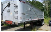
2008 EAST SMOOTH SIDE 28' ALUMINUM **DUMP TRAILER.** Aluminum Frame, 11x24.5 Tires, Air Ride, Needs Suspension Work, \$22,500.
