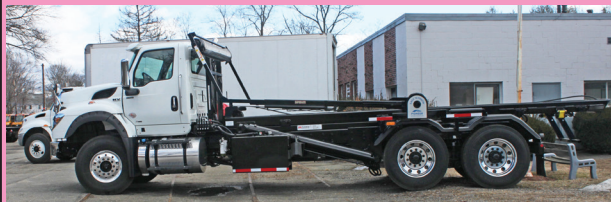
2020 INTERNATIONAL HV Roll-Off. 475 HP, A26, Automatic, 52K Rears, 22K Fronts And Rudco 75,000 LB Roll-Off Hoist.
