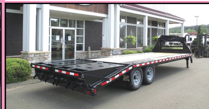
SURE-TRAC 15K DECKOVER GOOSENECK TRAILER. 8' 6" x 20 + 5' Beavertail, 32" Deck Height, Spring Assist Flip Over Ramps, #296436
