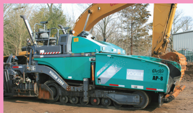
2010 VOEGLER VISION 5200-2. Crawler Asphalt Paver, #07740075, Cummins QSG 6.7, Rubber Tracks Carlson EZIV-1019, 10'-19' Hyd Ext Screed, Asking $35,000
