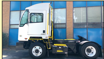
2020 AUTO-CAR ACTT42, SINGLE AXLE HYDRAULIC SPOTTER, CUMMINS B6.7L ENGINE, ALLISON 3000 SERIES TRANS. #190264
