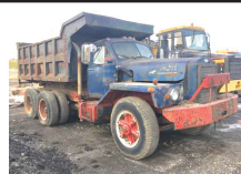
1955 MACK B81 TANDEM AXLE DUMP TRUCK. 237 with Jake Brake, 20 Speed Quadbox Transmission, 58K Rears. Great Farm or Site Truck. $4,500
