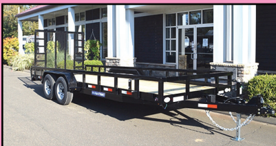
SURE-TRAC 9.9K OPEN LANDSCAPE TRAILER. 7' x 20', Steel Frame Pressure Treated 2 x 6 Decking, Spring Assist Rear Ramp, #308319
