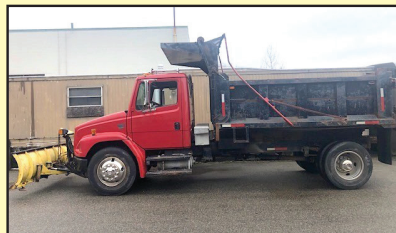
1998 FREIGHTLINER FL70, 33,000 GVW, DIESEL, 6SPD. TRANS., 12' DUMP W/ PLOW, 190K MILES, 12,000# FRONT / 23,000# REARS.
