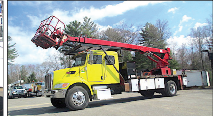
2008 PETERBILT 340: PACCAR PX8-300HP, 123K MILES, EXHAUST BRAKE, ALLISON 3500 RDS AUTO, 36K GVW, 5.26 GEARED RATIO, LOCKING DIFF, AIR-RIDE SUSP., 11R 22.5 TIRES, AIR-BRAKES/SEAT, A/C, PTO, ELLIOTT ECH-3-70 SIGN CRANE, 70' REACH, WINCH, HITCH REC., PINTLE $38,000
