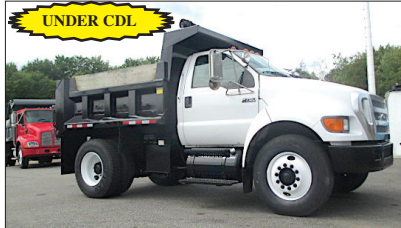
2007 FORD F-650: CAT C7-230HP, ALLISON 3500 RDS AUTO, 26K GVW, SPRING SUSP., LOCKING DIFF., 11R 22.5 TIRES, DBL FRAME, AIR-BRAKES, A/C, PTO, 9' STEEL DUMP, 2 CHUTES, PINTLE REC. $36,000
