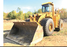
CATERPILLAR 980C. 3406, Powershift Transmission with 4 Speeds Forward and Reverse, 29.5-25 Tires, 5 Cubic Yard Bucket, Good Condition, Work Ready. $37,500
