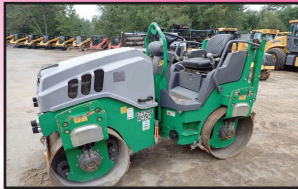
2016 HAMM HD12VV: 619 Hours, 48" Smooth Double Drum, Vibratory, Drops, 3 Cyl Kubota D1703, 24 Hp, 6k Lbs, stk#CO692, $19,900
