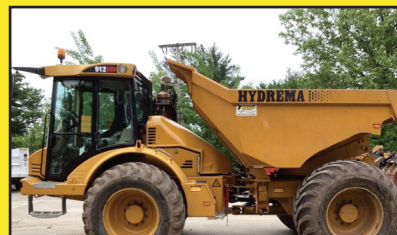
(2) 2021 HYDREMA 912HMS 22K LB CPTY, A/C, 141HP CUMMINS DSL, 180° MULTI-TIP 7.3CY DUMP BODY, AUTO-TIP SPD ADJ, MULTI-JYSTK CTRL, AUTO LUBE, 800/45-30.5 RBR, 800+ HRS STARTING AT $175,000
