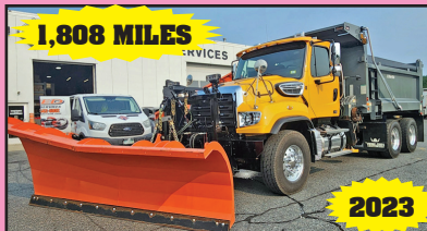
2023 FREIGHTLINER 114SD DUMP W/Plow And Wing. 470 HP, Allison 4500, 20 F/A, 46 R/A, Viking-Cives Equipment, 1,808 Miles.
