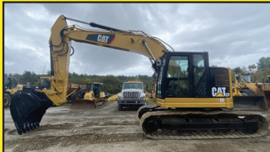
2016 CAT 325FLCR A/C, 18'8" BOOM, 9'6" STK, TEFFRA HYD Q/C, 48" BKT, LONG UC, ZERO TAIL, 32" TBG PADS, 4774 HRS $139,000
