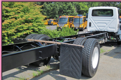
2023 INTERNATIONAL CV 515 CAB & CHASSIS 4X2. Allison Auto, 22,500 LB GVW, Air Ride Suspension, Wheelbase for a 14' Body. Call For Price
