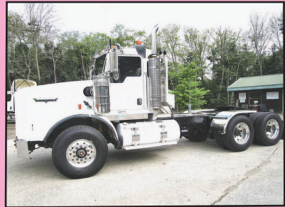
2004 KENWORTH T800W. CAT C-15 @ 550 H.P., Full Double Frame, 20F + 46R 2 Speed Rears, 3:90 & 5:38 Ratios, 11R24.5 Rear, 425 22.5 Front, 830K Miles, $75,000.
