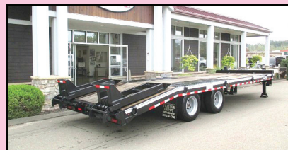
CAM SUPERLINE 51.7K HEAVY DUTY DECKOVER. 8' 6" x 25', 20 Flat + 5' Beavertail, Nominal 2" Oak Deck, 35" Deck Height, #538214
