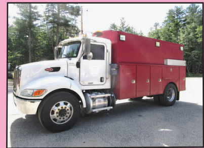
2014 PETERBILT 337. Paccar PX7 300HP, 26,000 GVW, Air Ride, 10F + 16R On Air Brakes, 138K Miles, Hours: 6360, 6 New 11R22.5 Tires, Curry Utility Body With Compressor, $60,000.
