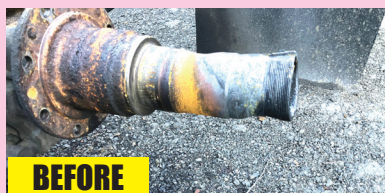
TRUCK DRIVE SPINDLE REPLACEMENT WELDED IN PLACE
