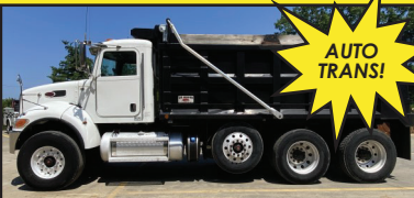
2019 PETERBILT 348 8X4 TRI-AXLE PACCAR 6CYL 380HP DSL, ENG BRAKE, DANA D46-170 DRV AXLES, 5.25:1 AXLE RATIO, 70K LB GVWR, AIR RIDE CAB, ALUM OUTER WHLS, STEERABLE AIR LIFT PSHR AXLE, CHALMERS SUSP, 218" WB, 16'6"L x 5'H STL BDY, 200K MI $159,000
