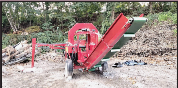
FIREWOOD PROCESSOR. AUTOMATED, 3 STRAND LOG TABLE, IN-FEED CONVEYOR, HYDRAULIC CHAINSAW 25" BAR, 4 WAY SPLITTING BLADE (6 WAY AVAILABLE), OUT-FEED CONVEYOR, 30 TON SPLIT FORCE, 27 HP MOTOR, 32 GPM PUMP, $14,500. 401-363-1508
