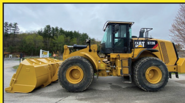
2012 CAT 972K EROPS, A/C, 7CY PIN-ON BKT, JYSTK STR, AUTOSHIFT, RIDE CTRL, AIR RIDE ST, REAR CAM, 26.5-25 TIRES, 2646 HRS $139,000
