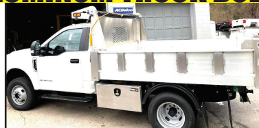
DURA MAG ALUMINUM DUMP BODIES Complete Sub-Frame, Power Pac, LED Lights.
