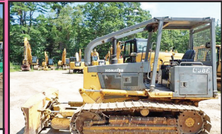
1999 KOMATSU D38E-1: 4,745 Hours, 6-Way Blade, Orops W/ Sweeps, Joystick Steer, 17.5k Lbs, stk#DZ996, $23,500
