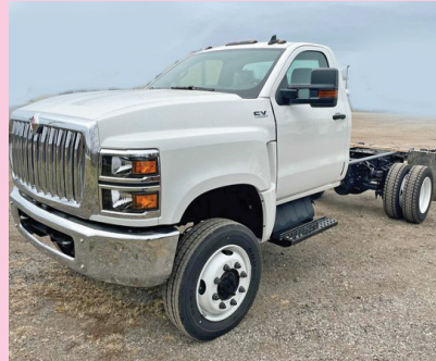
2023 INTERNATIONAL CV. 22,500 GVW, Air Ride Suspension, Allison Auto, 2 Wheel Drive, Wheelbase For a 14' Body. (file photo)
