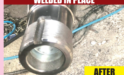
TRAILER SPINDLE REPLACEMENT WELDED IN PLACE
