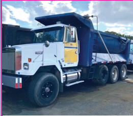
1994 AUTOCAR TRI AXLE DUMP TRUCK: 3406C CAT, 8LL, 46/18, Has Been Rolled Over, Salvage Title, 11x24.5 Tires @ 90% On Alum. Rims, Drives, A Lot Of Good Parts, 17' Rock Body W/ High Lift Gate, Will Part Out, $10,500.
