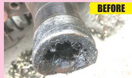
TRAILER SPINDLE REPLACEMENT WELDED IN PLACE
