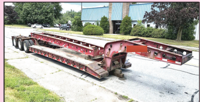
1998 FONTAINE, MODEL. 50 Ton, Detaches At Both Ends, 25' Flat Level Deck - 20" Loaded Deck Height, 25' Beam Deck Insert, 20" Loaded Deck Height, Non Ground Bearing, Air Ride, Boom Trough & Deck Cut Out, Lift Axle, Outriggers, Aluminum Wheels, Strobe Lights. Call For More Information.
