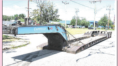
2007 TALBERT. 55 Ton, Flat Level Deck, 25' 6" Deck, Tri Axle, Air Ride, Non-Ground Bearing, Set Up For 4th, Air Lift On Third, Working Daily, One Owner. Call For More Information.
