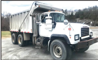
2003 MACK T/A DUMP. Mack E7- 350 Hp, 8LL, 20 Frt Axle on 425 Floats, 46 Rears, 11R22.5, Camelback Spring Susp, Dbl Frame. 14' BENSON Aluminum Body, 61" Sides, Elect Tarp, Pintle Plate, 188,633 Miles #065180, $34,500.
