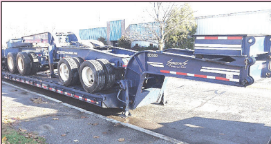
2012 ITI DDX100 70 TON 2+2+3 HYDRAULIC EXTENDABLE STEERABLE TRAILER. Air Ride. Comes With 10' Flip Up Gooseneck Ext, Self-Contained Power Unit, 30' Deck, 8' 6" Wide, JP40 Tandem Axle Jeep, B80 Tandem Axle Stinger With Pin On 3rd Axle. Wireless Remote, Super Singles. Call For More Information.
