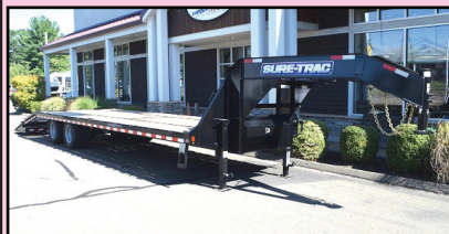
SURE-TRAC 22.5K LOW PROFILE DECKOVER GOOSENECK. 8' 6" x 25' + 5' Beavertail, Bi-Directional Springs In Ramps, Oil Bath Axles, #372758
