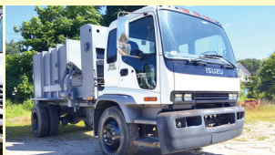
2007 ISUZU FVR: UNDER CDL, AIR-BRAKES, 111K MILES, ALLISON AUTO, MOUNTING 2011 10YD NEW WAY SIDE LOADER W/ TIPPER. CHASSIS BLASTED & PAINTED, BODY PAINTED YOUR CHOICE OF COLORS.
