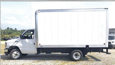
NEW E350 DURA CUBE 14' VAN BODY. Pull Out Ramp, Roll Up Rear Door, Step Bumper, V8 Gas, Pass Thru Door, E-Tracks, #21025
