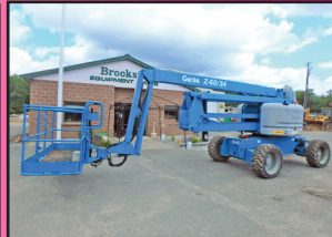
2012 GENIE Z60/34: 2,943 Hours, 60 Ft Knuckle Boom, 34 Ft Horizontal Reach, 4x4, 8 Ft Basket, 4 Cyl Perkins Diesel, Jib, stk#AE018, $29,900
