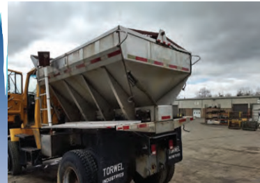
10ft Torwel, front discharge, with stainless steel hydraulic tank
