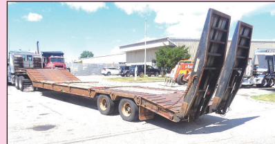
2008 PITTS LB35 , 35 Ton, Drop Deck With Beaver Tail And 8' Hydraulic Ramps, Self-Contained Hydraulic System, 102" Wide, Roll Down Landing Gear, Tool Boxes, Original Paint, 1 Owner, Very Good Condition. Call For More Information.
