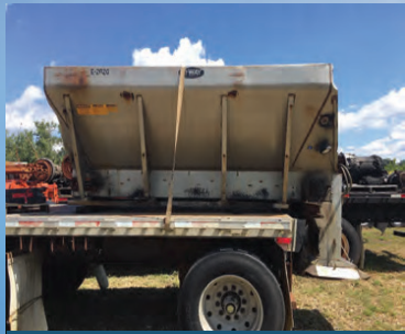
10ft Highway Equipment Co. Model E2020-10, rear discharge, top RH side of tub bent
