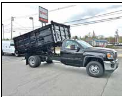
2016 SIERRA 3500 12FT KNAPHEIDE LANDSCAPER DUMP BODY. 4x4, Solid Sides, Curd Side Door, HD Hoist, 6.0L V-8, Plow Prep, Trailer Brake, Power Locks & Windows, #G16122
