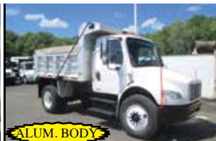
2005 FREIGHTLINER M2 BUSINESS CLASS, CAT C7 230HP., 123K MILES, ALLISON 3500RDS AUTO, 26K GVW, SPRING SUSP. W/ HELPERS, 6.14 GEARED RATIO, LOCKING REAR DIFF., SINGLE FRAME, AIR BRAKES, AIR SEAT, A/C, PTO, 10' ALUM. J&J DUMP, 1 CHUTE, AIR GATE, AUTO TARP, PINTLE. $37,000
