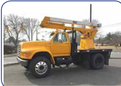
1996 Ford F800 Bucket Truck. Cummins diesel, Allison auto, only 37K miles, 36' reach, #T0404AA, $21,900
