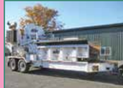
2006 Bandit Beast, 765 Original hours on the machine, Model 2680, C-9 Cat Diesel @ 300 HP, Pt Tech HPTO 12 Clutch, Remote control, Magnetic head pulley, All new tips installed less than 40 hours ago, Comes with 3 sets of screens. In Excellent condition, and ready to grind.
