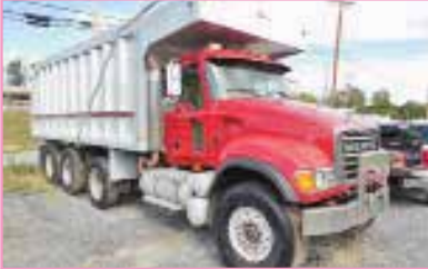
2007 MACK GRANITE TRI AXLE DUMP TRUCK, 8LL TRANS, E7427 ENGINE, 58K LB REARS, LESS THAN 200K MILES, CAMEL BACK SUSPENSION FLOATS ON FRONT, 21' BENSON ALUMINUM BODY. CALL FOR MORE INFORMATION.
