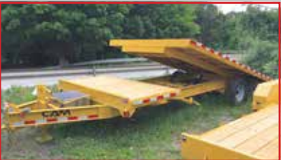
24' CAM Deck Over Split Tilt model 7CAM824DOSTT, 102" wide, knife edge approach plate, stake pockets and rub rail, 8 D rings, 12K jack, aluminum tool box, wireless remote w/ power up & down, $8,995
