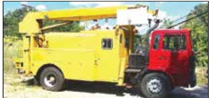
1984 MACK MS250P. ALTEC 15,000 LB CRANE, AUGER WITH 2/BITS, BUCKET WITH UPPER CONTROLS, POLE CLAW, EVERYTHING WORKS, $9000. 508-560-2484
