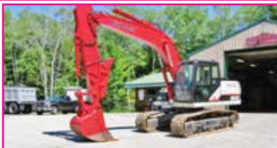
2012 Linkbelt 160X2. 2500 hrs, hydraulic thumb, long stick, 36" Escalator bucket, 24" shoes 8'6" wide, pattern changer, $80,000.
