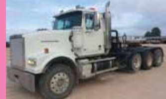
2013 WESTERN STAR 4900 Detroit DD15 14.8L Engine, Engine Brake, Eaton Fuller 18 Speed Manual Transmission, 251" Wheel Base, 18,180 lb. Front Axle, 43,000 lb. Rears, Air Ride Cab, Air Lift Pusher Axle, Double Frame $89,000
