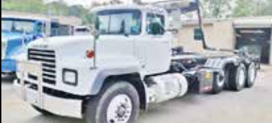
2003 MACK TRI AXLE ROLL OFF. 76,650 lb GVW, Galbreath 60K lb Hoist, Mack 350, 8LL, heavy specs. Package comes with 4 30 and 1 20yd, owner operator truck, maint. records, not junk, $79,500. 401-828-7274
