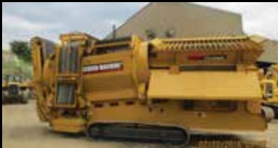
2014 SCREEN MACHINE 612T YANMAR DSL, 5'10" FOLLER BELT, 36"X9' REAR DIS CNV, RMT CNTRL 24"X25' SIDE DIS, 42" X7' UNDER SCREEN CONV. POR
