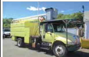
2007 INTERNATIONAL 4300 DT466, 245HP., PRE-EMISS., 7SPD., 26K GVW, SPRING SUSP. W/ HELPERS, SINGLE FRAME, AIR BRAKES, PTO, DUAL HYD. OUTRIGGERS, 11' STEEL SOUTH CO CHIP DUMP, 1-PACK, ARIEL LIFT AL60, 60' BOOM, BOOM TIP CONTROLS, PINTLE. $36,000
