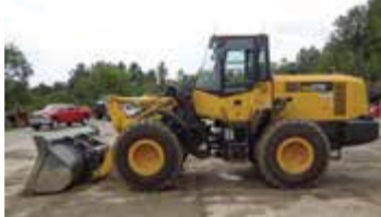
(2) 2015 KOMATSU WA270-7'S EROPS, AC, 20.5 RADIALS, JRB, 3.0 CY BUCKET W QC, REAR VIEW CAMERA $135,000 EACH
