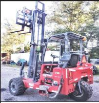
2014 MOFFETT M55.4P FORKLIFT. Piggyback, 4 Way Ext. Reach, 5500# Capacity, + Sideways Driving. Only 960 Hours, Carry On The Rear Of Truck/Trailer, Excellent Running Condition! \$38,500. Call Jesse, 401-855-1178
