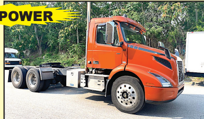
2019 VOLVO VNR64T300-D13, 500HP, 12SPD. I-SHIFT, AUTOMATIC, 14,600# FRONT / 46,000# REARS, AIR-RIDE, 282K MILES. #210088A
