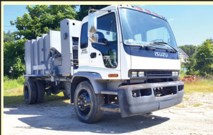
2007 ISUZU FVR: UNDER CDL, AIR-BRAKES, 111K MILES, ALLISON AUTO, MOUNTING 2011 10YD NEW WAY SIDE LOADER, W/ TIPPER, CHASSIS BLASTED & PAINTED, BODY PAINTED YOUR CHOICE OF COLORS.
