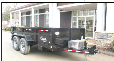
CAM SUPERLINE 13.2K HEAVY DUTY LOW PROFILE DUMP TRAILER. 6'9" x 12', Slipper Spring Suspension, 3 Way Combo Gate, #522858
