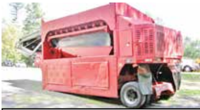
2005 EXTEC 4500. 1134 hours, 6' X 12' deck, Deere 4 cylinder, 54" X 32' conveyor, 2" screen, $47,500.
