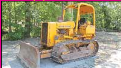
1984 John Deere 450E Crawler Dozer. new tracks and chains with ZERO hours, runs good, 15630 lb machine, 4 speed hi/lo transmission, 202 cu in diesel, 57HP. $15,500
