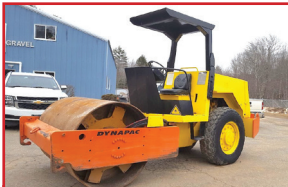
1989 DYNAPAC CA151-1D. Vibratory Compactor, 3,867 Hours, 66" Smooth Drum, #2657, $26,000
