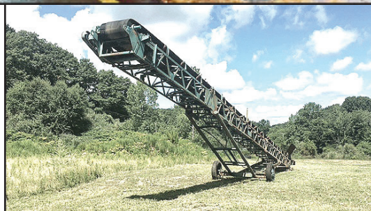
YELLOW STACKING CONVEYOR. 30" X 55 Ft., 42" Wide X 24" Deep Truss, 2" X 3" X 1/4" Angle, 10 Hp., 240/480 Volt, 3 Phase Motor, Solid Conveyor, $6,800. Gales Ferry, CT 860-460-0767
