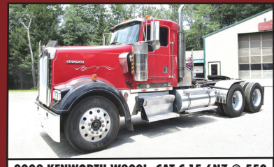
2002 KENWORTH W900L. CAT C-15 6NZ @ 550 H.P., 186K Miles (Verified), Reman 18 Spd, 4:56 Ratio, 13.2F + 46R, 52 lb. New Way, Dbl Frame, New Tires, $105,000.
