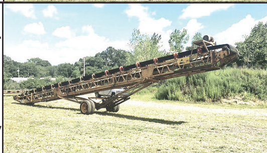
BLUE 30" X 56 FT. RADIAL STACKING CONVEYOR. 42" Wide X 24" Deep Truss, 2.5" X 2.5" X 1/4" Angle, 10 Hp., 240/480 Volt, 3 Phase Motor, Folding Upper Section, $7200. Gales Ferry, CT 860-460-0767
