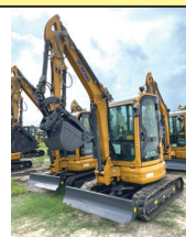
XCMG XE35U 9,200lb Unit, Yanmar Engine, Dual Aux Hydraulics, 5yr/ 5000hr Warranty
