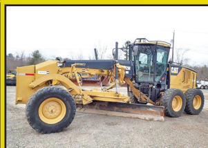
2011 CATERPILLAR 12M: 8,902 Hours, Cab W/ A/C, 14 Ft Mold Board, Scarifier, 6 Cyl Caterpillar C6.6 Turbo, stk#GR077, $89,950
