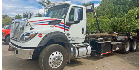
2019 INTERNATIONAL HV ROLL-OFF. Galbreath 75000 Hoist, Allison 4500 Trans, 52K Rears, 20K Front, 130K Miles.
