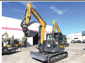
XCMG XE80U 19,500lb Machine, 73HP Kubota, Dual Aux Hydraulics, 5yr/ 5000hr Warranty
