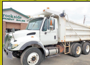
2005 INTERNATIONAL Workstar 7500: 10 Wheel, 13 Ft Steel Henderson Body W/ 3 Chutes, IH HT570, 310 HP, Allison Auto, Hendrickson Rubber Block Suspension, Hitch W/ Air & Electric, 12K F, 40K R, stk#TK063, $49,500
