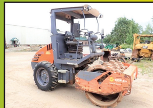
2015 HAMM H51: 1,439 Hours, 54" Smooth Drum W/ Padfoot Shell Kit, Drum Drive, Vibratory, 4 Cyl Kubota Turbo, 73 Hp, 11K Lb + Shell Kit, stk#C0557, $43,500
