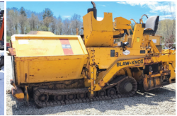
BLAW-KNOX PF-410 PAVER. John Deere 4039 Diesel Engine, 6128 Hr, 13" Steel Tracks W/ 17" Rubber Pad Tracks, Rakes, Belts & Hoses Included, 8' Open To 11' Hopper. 102"W X 178"L X 118"H, $12,000
