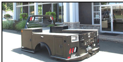
TM DELUXE TRUCK BED. Fits Any Chassis Cab 60" CA, 6 Lockable Tool Boxes, Used CM Truck Bed, 7' x 9'4", #00179744, $4,500
