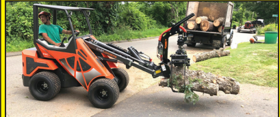
CAST 23T. 23HP Kubota Diesel, Extendable Boom, Aux Hydraulics
