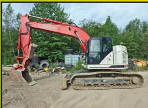
2016 LINK-BELT 235 X3 SPIN ACE: 1,530 Hours, 42" Digging Bucket & 62" Cleanup Bucket W/Wrist, Craig Hyd. Thumb & Coupler, A/C, Reduced Tail, 9'10" Wide Blade, 2 Speed Travel, 4 Cyl Isuzu Turbo, 57K LBS, Very Good U/C, stk#XC346, $139,500
