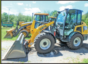
2017 GEHL AL650: 333 Hours, 1 Yard, Cab, Hyd Coupler W/ 3rd Valve, 4 Cyl Yanmar Turbo, 3 Speed, 9.5K Lb Size Class, Stk#LO190, $49,500
