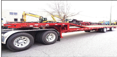
2012 TARASPORT 50' Tandem Spread Axle Step Deck Trailer, Sandblasted & Painted. New Brakes, Seals, Bearings, Hubcaps, Flaps & Decals. Front And Rear Pull Outs To Extend Trailer, Spring Assisted Ramps From Lower Deck To Upper Deck, 12' Alum Pull Out Ramps, Air Ride, 10' Upper Deck, 40' Main Deck, 102" Wide, 22.5 Lo Pro Tires, Excellent Shape. Call For More Information.
