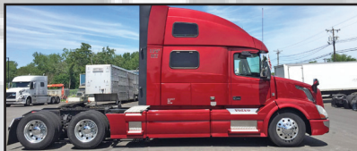
2016 VOLVO VNL64T780 77" Sleeper. 6x4, D13 500 HP, I Shift 12 Spd, Engine Brake, 40K R/A, 472K Miles, stk#U603VN
