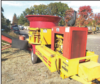
HAYBUSTER HD8 TUB GRINDER. Just Refurbished! New Clutch, New Injectors In John Deere 4039T Engine, New Hydraulic Motors, New Hammers, New Exhaust, And More, $29,500. Call Jesse, 401-855-1178
