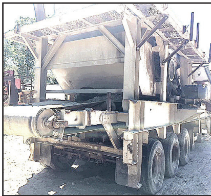
1989 NORDBERG 1352 OMNICON PORTABLE CONE CRUSHER: S/N: 5202-577, Simplicity 6203, 6' X 20', Triple Deck Horizontal Screen, 200 HP, 480 Volt Soft Start Electric Motor, Three Axle Nordberg Carrier, $98,000 OBO. Chris, 860-460-0767 Or Chm@Terrafirmas.com
