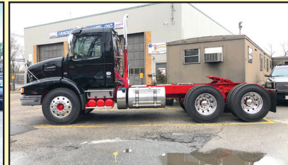
2019 VOLVO VDH64BT300-D13,, 500HP, I-SHIFT TRANS., 14,600# FRONT/ 46,000# REAR T-RIDE, HYD. WET-SYSTEM. #180228
