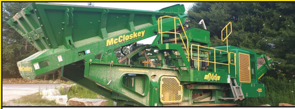
2017 MCCLOSKEY C44 CONE CRUSHER TELSMITH 44SBS 44" CONE, AUTO ADJUST, 7'x12' FDR, 42"x18' OVER FEED CONV, 42"x30' UNDER CRUSHER DISCH CONV $459,000
