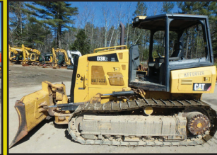
2012 CATERPILLAR D3K2 XL: 7,682 hours, 6-way blade, orops w/ heat, joystick steer, 16" pads, 4 cyl Cat C4.4 Acert turbo, 80 hp, 17.5k lb size class, stk#DZ120, $47,500
