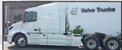
2020 VOLVO VNR64T640 61" Sleeper. D13-500HP, I-Shift 12 SPD AMT, Dual 150 Gallon Tanks, 221" WB, 40K R/A, stk#VN620
