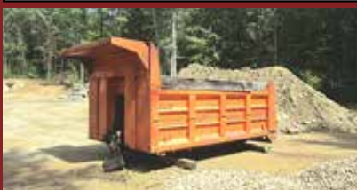
14' BIBEAU DUMP BODY, With Hoist, 48" Sides, 54" Gate, 1 Chute, Some Rust In Rear, $4000.
