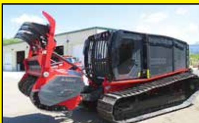
2017 PRINOTH RAPTOR 300 FORESTRY MULCHER. Cat C7.1, PTO Driven Head, Winch, Backup Camera
