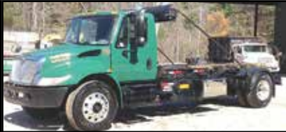
2007 INTERNATIONAL 4300 ROLL-OFF. Galbreath 25K Extended-A-Tail Roll-Off Hoist W/Short Stops, Int'l Eng., 6 Spd. Manual, 12F/21R, Pioneer HR1500 Tarper, 184K Miles. Too Many Extra's To List! $43,500. Rick 978-423-6267
