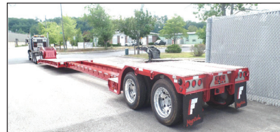
IN STOCK - 2025 FONTAINE LXTN40. 40 Ton Extendable, 34' Closed - 60' Open. Also Available 29' Closed - 50' Open. Tandem Axle, Set Up For 3rd, Air Ride, Non Ground Bearing, 102" Swing Clearance, 20" Deck Height, Alum Wheels. In Stock, No Waiting. Available In Manchester NH and At The Factory In Springville AL. 3rd And 4th Axles Available. Call For More Information.
