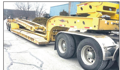
2017 LIDDELL 60 TON DSR. 4 Axle, 26' DSR Deck, 9' Wide, 8'6" Bogie, 26' Beam Deck, 4th Axle, Alum Wheels, Gooseneck Extension, Power Pack, Excellent Shape, Call For More Information.
