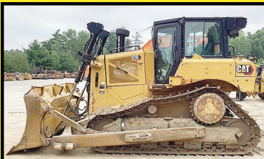
2020 CAT D6 128" HYD SEMI-U ANGLE BLADE, 24" METAL TRACKS, PULLBAR, 8200 HRS $149,000
