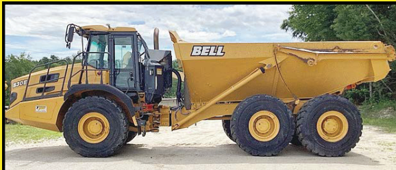
2022 BELL B30E A/C, 6X6, ENG RETARDER, MERCEDES DSL, TAILGATE, 23.5R25 RADIALS, 3900 HRS $159,000
