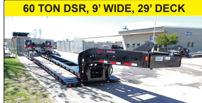
IN STOCK - 2027 FONTAINE MAG60 DSR. 9' Wide, 29' Deck, Dual King Pin With 81 And 102 Inch Radius, 137 Inches With Flipbox, 54.5" Axle Spacing, Tri Axle, Set Up For 4th, Air Ride, Alum Wheels, Set Up For Wet Line, 275 Rubber. Call For More Information.
