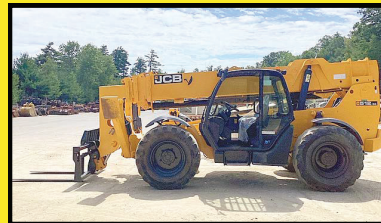
2016 JCB 512-56 56' LIFT HT, EROPS, AUX HYD, MNL Q/C, 48" FORKS, FRAME LVL, 74HP TIER-4 FINAL DSL, 4- SPD TRANS, OUTRIGGERS, 17.5-25 L2 TIRES, 4341 HRS $75,000
