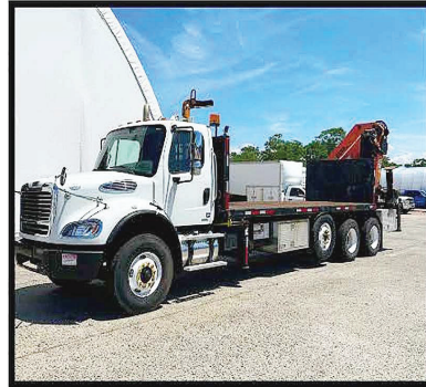
2009 FREIGHTLINER BUSINESS CLASS M2 112 35,740 mi., Detroit diesel, Allison auto, engine brake, equipped with Palfinger PK72002 knuckle boom. Comes with pallet forks. Used for 1 project and no longer needed . . . . . $105,000 OBRO
