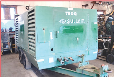
1990 SULLAIR 750Q. Oil-Flooded Rotary Screw Air Compressor For Heavy Duty Work, CAT Engine, 750 CFM, $7,500
