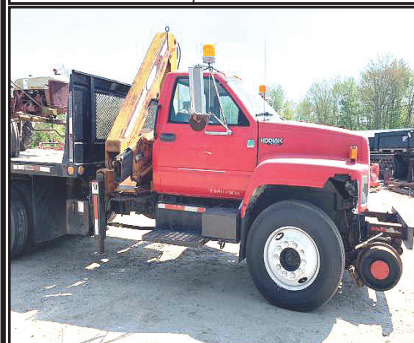
1993 CHEVY KODIAK RAILROAD TRUCK. CAT Enginem, 6 Speed Manual, 79xxx Miles, Knuckle Boom Crane Tico 771H Works Great, Has 2 Outriggers, Rear Pintle Plate, Flatbed 16.5 Ft. Long, Drop Axle, 4 New Tires, New Front Tires, New Rear Springs, $6200. 603-231-1767
