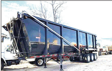
2021 GALLEGOS 42' FRAMELESS DUMP TRAILER , 96 Yard, Tri Axle, Hendrickson Air Ride Intraxx, ABS Brakes, Lift On Front Axle, Cramaro Flip N Go Canvas, Steel Wheels, LED Lights, Barn Door. Call For More Information.
