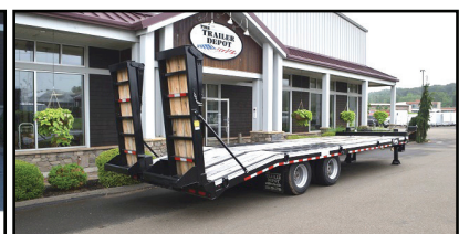
CAM SUPERLINE HEAVY DUTY 51.7K DECKOVER. 8'6" x 27', 22" Flat + 5" Beavertail, 102" Overall Width, 35" Deck Height, #520128
