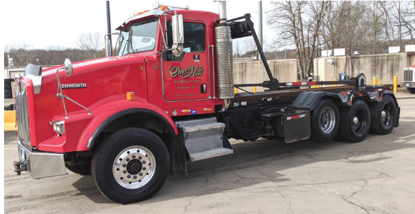
2004 KENWORTH T800 Roll-off , 600,000 miles, 20K Front, 40K Rears, Fixed Pusher Axle, 8 LL Eaton Fuller (1yr old), C15 475 Engine, Galbreath Hoist, Auto Tarp, Auto Can Lockers. Asking $59,000.
