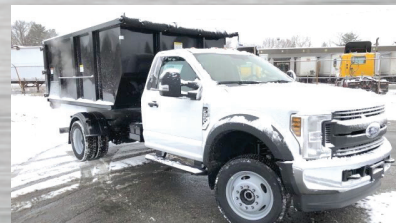
2019 F550 HOOKLIFT 4X4. 15,000 lbs Hoist, V10, Limited Slip Axle, Running Boards, Package Upgrades, Snow Prep, Heated Mirrors, #194832
