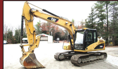
2008 CAT 312 DL. 8' 6" Wide, 36" CAT Bucket, Common Pin Hyd. Thumb, 7018 Hours, 4 New Injectors, $58,000.
