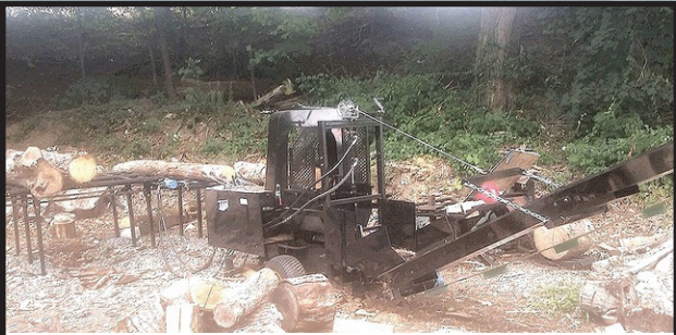
FIREWOOD PROCESSOR. ALL HYDRAULIC, CHAIN DRIVEN LOG TABLE, 25" HYDRAULIC STIHL CHAINSAW, 30T SPLITTING FORCE, FEED AND DISCHARGE CONVEYORS, NEW 20 HP HONDA MOTOR, LIKE NEW, $7,800. 401-390-4976
