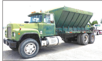
1990 MACK RD688S . Cummins, 400 HP, Eaton Fuller, 8LL, Camelback Spring, 234" Wheelbase, Double Frame, 18K Front, 46L Rears. Call For More Information.
