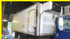
2007 Morgan Reefer Body 22' x 102", Carrier unit with stand by, 230V, 3 phase, 60 HZ, E-track, 2 side doors, roll up door, walk ramp, excellent cond, $7,000 Cash & Carry
