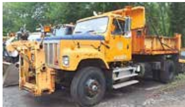
2002 Int'l 2574 S/A dump, 9spd central hyd., 300 Cum. w/Jake, single wing set up, 98k mi., pwr revers frt hook up
