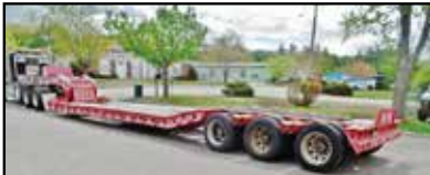
1997 FONTAINE 50 TON ROLLER/PAVER STYLE TRAILER, NON GROUND BEARING, AIR RIDE, 25' LEVEL DECK, 5' RAMP, LOADABLE OVER TRI AXLE BOGIE. CUT OFF FRO BOOM TROUGH. 102" WIDE, OUTRIGGERS AND D-RINGS. HUB PILOTTED WHEELS. 2 CHAIN LIFTS, FRONT PAVER RAMPS, STROBE LIGHTS, ONE OWNER, RECENT PAINT. CALL FOR MORE INFORMATION
