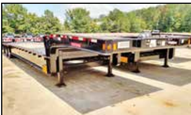
NEW 2016 FONTAINE XCALIBUR EXTENDABLE DROP DECK TRAILER. ADJUSTS FROM 53' TO 72'. TRI AXLE, UPPER DECK 10'6" LONG, 59" HIGH, LOWER DECK 42' 6" LONG, 34" HIGH. 2 SPEED LANDING GEAR. 235/75 RUBBER. WINCH TRACK AND WINCHES. CALL FOR MORE INFORMATION.
