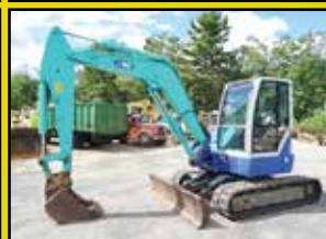
2007 IHI 80NX3: 3,778 HOURS, AUX HYD, CAB W/ A/C, 87" BLADE, MECH COUPLER, 2 SPEED, 4 CYL ISUZU, REDUCED TAIL SWING, SWING BOOM, COMES W/ 23", 28" AND 12" DIGGING BUCKETS AND 48" CLEANUP BUCKET, 18.5K LB SIZE CLASS, STK#XC378, $36,900
