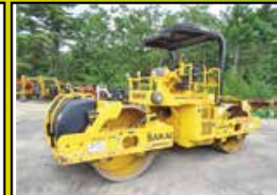
2009 SAKAI SW650 II: 3,487 HOURS, 78" SMOOTH, DOUBLE DRUM, VIB., OROPS, 6 CYL DEUTZ TURBO, FRONT & REAR WATER SYSTEM, 28K LB SIZE CLASS, STK#CO16, $37,500
