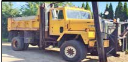
1987 INTERNATIONAL PAYSTAR 5070. Single axle, 4WD, 8LL, new tires, cab very good, set up wing sander plow, 6V 92 Detroit. Many new parts, no rust, $16,500 OBO. 413-575-2069
