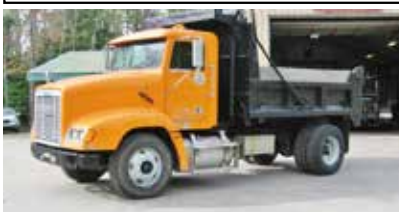
1998 Freightliner FL112. M11 Cummins @ 280 H.P., 9 spd., 32,000 G.V.W., 11' Everest heated body, pintle hook, 11R22.5, 504K miles, cold AC, $10,000.
