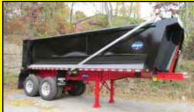
2016 26' RHODES STEEL DUMP, 70,000#, SINGLE POINT, HIGH-LIFT GATE.
