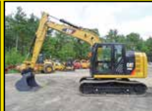
2012 CATERPILLAR 312E: 2,723 HOURS, 48" BUCKET, AUX HYD, HYD GEITH COUPLER, VERY GOOD U/C, 2 SPEED, A/C, 4 CYL CAT TURBO, 33K LB SIZE CLASS, STK#XC213, $99,500
