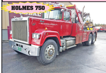
HOLMES 750 1978 MACK SUPERLINER RWS786LST w/Holmes 750 Wrecker. E6-2V 300 HP, 6 Spd., Engine Brake, 232" WB, 12K F/A, 38K R/A, 168K Miles, stk#38941, $27,500
