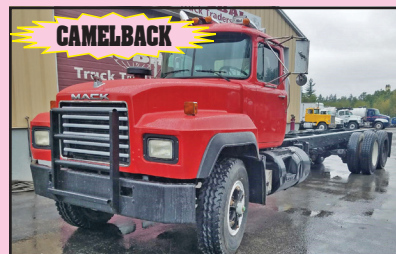
CAMELBACK 1995 MACK RD688S C&C. EM7 350HP Diesel, 9 spd OD., 290" WB, Jake Brake, T/A, 18K F/A, 44K R/A, 265K Miles, Stk#22292, $24,900.
