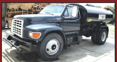
1995 Ford F-750. 5.9 Cummins, 6 Spd, 30,000 G.V.W., 2000 Gal Tank With Front Spray Head, $14,000.
