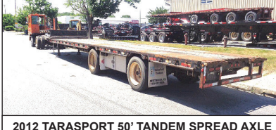
2012 TARASPORT 50' TANDEM SPREAD AXLE STEP DECK TRAILER , With Front And Rear Pull Outs To Extend Trailer, Spring Assisted Ramps From Lower Deck To Upper Deck, 12' Alum Pull Out Ramps, Air Ride, 10' Upper Deck, 40' Main Deck, 102" Wide, 22.5 Lo Pro Tires, Excellent Shape, Call For More Information.
