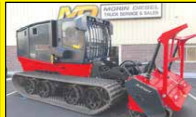
PRINOTH RAPTOR 300R FORESTRY MULCHER, Cat C7.1, Hydrostatic Drive, Pto Driven Head, 3.7Psi Of Ground Pressure
