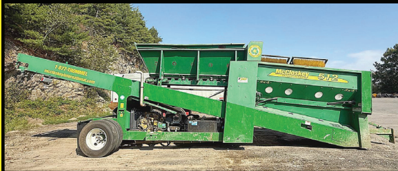
2020 MCCLOSKEY 512A 5'X12' TROMMEL, 3-5CY CPTY, 1/2" OR 3/4" SCRNS, 100HP TIER-3 DSL, PINTLE HITCH, 11R22.5 TIRES, 1621 HRS $149,000
