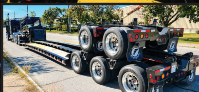
2027 FONTAINE 80/100 TON DROPSIDE LOWBED. 30' DECK, 9' WIDE, MODULAR, PIN ON AXLES, 7 POSITION HYDRAULIC DETACHABLE GOOSENECK, AIR RIDE TRIDEM BOGIE, ALUM WHEELS, NON GROUND BEARING, TOOL BOXES, 603-641-8608
