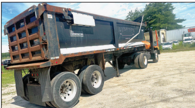
2008 KRUIZ 26' DUMP TRAILER. 24.5 Rubber High Lift Gate, 1/4" Hardox, 70K Lb. Suspension, Electric Tarp, 1 Owner, Very Good Condition, Price $27,500. Call For More Information.
