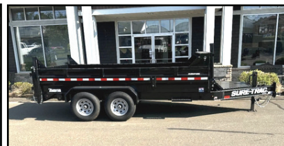
SURE-TRAC PRO SERIES 15.4K TELESCOPIC DUMP TRAILER. 7' x 14', 24" Rigid Side Walls, Slipper Spring Suspension, #454380
