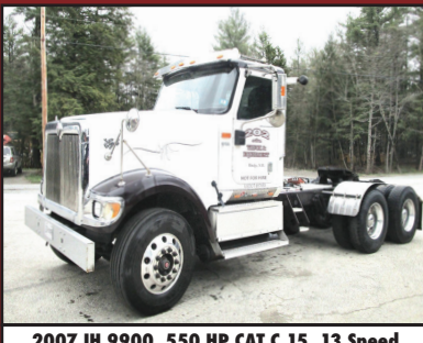
2007 IH 9900. 550 HP CAT C 15, 13 Speed, 12,000 Lb Front Axle + 40,000 Lb Full Locking Rear Axles On Air, Wet Line, Single Frame, 205 WB, 550K Miles, This Has Been Our Spare Truck For The Last 3 Years, New $5000 ECM Just Installed, Needs Nothing, $37,500.
