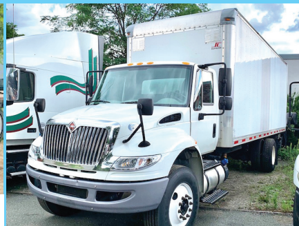
2015 INTERNATIONAL 4300 24' VAN. Cummins ISB, 240 HP, Allison Auto, Spring Suspension, Under CDL, Alum. Lift Gate, New Tires, 238K Miles, Southern Truck.
