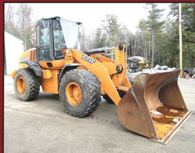
2013 CASE 721F. 4600 Hrs, 3.5 Yd, Q/A Bucket, JRB Coupler, 3rd Valve, 50% Matched Michelins, $74,000.
