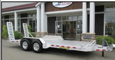
ALUMA 14K EQUIPMENT TRAILER. 6' 10" x 18", 79" x 224" Bed, Rubber Torsion Axles, #214248
