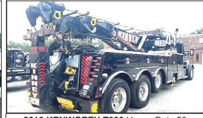
2016 KENWORTH T880 Heavy Duty 50 Ton Century/Rotator Slider , 5 Winches, 550 Cummins, 18 Speed, 52K Rears, Air Ride, 20K Front, 20K Steerable Lift Axle, 56,000 Miles, Fully Equipped, Fully Loaded. Alum Wheels, Call For More Information.
