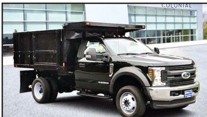
2019 F-550 XL 4WD DUMP BODY: 6.7L Power Stroke V8 Turbo Diesel, Remote Start, 19,500 GVW, stk#N8539
