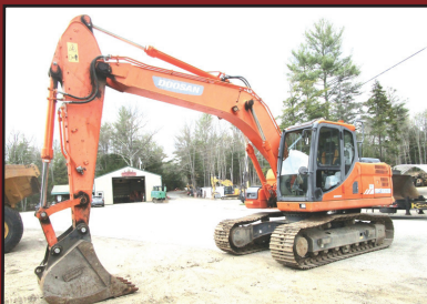
2014 DOOSAN DX180 LC-3. 8'6" Wide, Aux. Hyd., 36" Bucket, 39,000 Lbs., $77,000. Also Available Full Rotation Thumb, $7500.
