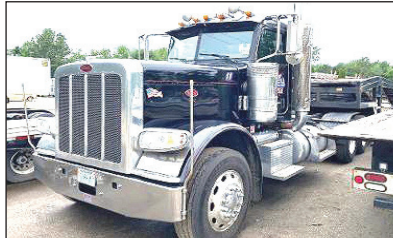
2014 PETERBILT 388 TRACTOR , 550 Cummins, 18 Speed, 46K Rears, Tandem Axle, Air Ride, Wet System, Alum Wheels, Loaded, 490K Miles, One Owner. Call For More Information.
