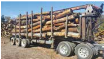
TRAILMOBILE TRI-AXLE. Air Ride, 3rd Axle Lift, 22.5" Tires on Steel Wheels, 35ft. x 8ft., 8 Log Bunks, Hood Log Loader w/Extendable Rotobec Rotating Grapple, $14,800.
