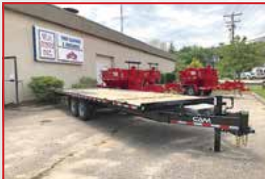
24' CAM SPLIT-TILT HD DECKOVER TRAILER. Model 8CAM824DOSTT, 18400 LB GVW, 13270 LB Payload Capacity, 102" Wide, Black
