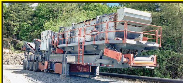
SUPERIOR P300 CLOSED CIRCUIT CONE CRUSHING PLANT. 6X20 TRIPLE DECK, MAKES 3/4" MINUS MATERIAL, NEW MANGANESE INSTALLED, ABSOLUTELY IN EXCELLENT CONDITION, JOB READY, $850,000. 941-960-6169
