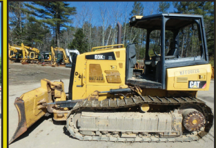
2012 CATERPILLAR D3K2 XL: 7,682 hours, 6-way blade, orops w/ heat, joystick steer, 16" pads, 4 cyl Cat C4.4 Acert turbo, 80 hp, 17.5K lb size class, stk#DZ120, $47,500
