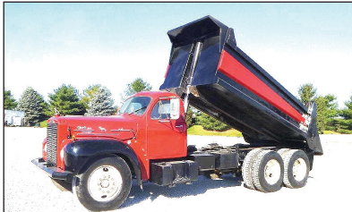
1959 MACK B753S DUMP TRUCK , Tandem Axle, 6 Cylinder, 5 Speed, Camelback Spring, 204" Wheelbase, PTO, 14' Box. Call For More Information.
