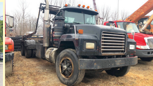
2001 MACK R MODEL : SHOWS 165K MILES, CHAGNON 22' 75K HOIST, PIONEER 4500 TARP, 8 SPEED FULLER TRANSMISSION. $17,500
