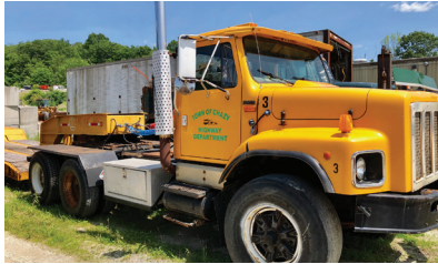
1995 IH 2674 Tandem Tractor. 400 HP N14, 13 Speed, 46K Rears, 20K Front, Dual Line Wet Line, $15,000
