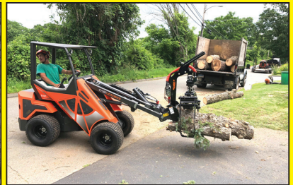
CAST 23T. 23HP Kubota Diesel, Extendable Boom, Aux Hydraulics
