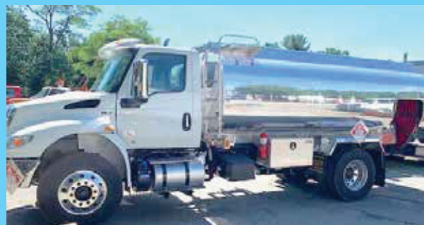
2020 INTERNATIONAL MV 2800 Gallon Amthor Tank. 33,000 GVW, Allison 3000 Transmission, Loaded.
