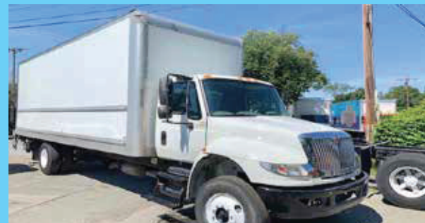
2015 IH 4300 26 FT Box and Gate. Non CDL, Cummins ISB, Air Brakes, Automatic.
