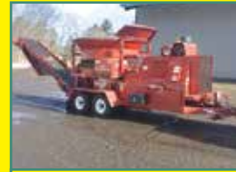
2009 Morbark Tub Grinder Model 950. Cat Diesel @ 210 HP. 3463 Hours. Remote control. Magnetic head pulley 3" hex screens Call for price
