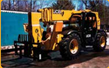
JCB 510-56 #58811 10k lb lift cap, 56' telehandler, cab heat & a/c
