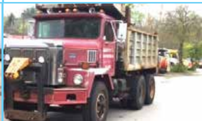
1988 IH PAYSTAR 205K Miles 315 Cummins 8L1 Transmission 18K Front 46K Rear Walking Beam Suspension 13 Ft 6 Inch Dump Body 11 Ft Wing Plow Included. A Bit Rusty And Needs A Bit Of TLC But An Oldie But Goodie. Sale Price $15,500.00
