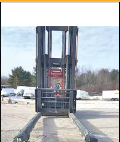
2002 TAYLOR TMH120 MARINE FORKLIFT. 20,000 lb Lift, 20 Ft Padded Boat Forks, Two Stage, Side Shift, Cummins 160Hp, 3 Speed, Air Brakes, 5000 Hours, $125,000. 207-240-5793
