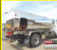
2017 HINO 338 OIL TRUCK. 2700 GALLON ALUMINUM DUEL COMPARTMENT TANK, 120K PSI FRAME, #8388
