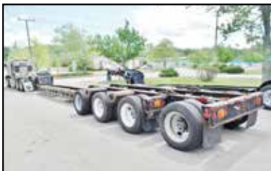
2000 FONTAINE 60 TON BEAM TRAILER, 3 AXLE WITH 4TH AXLE FLIP, AIR RIDE, 28" USABLE BEAM DECK, 60" AXLE SPACING, MODULAR DETACHES AT BOTH ENDS, 120" SWING CLEARANCE, LO PRO TIRES, STROBES, NON GROUND BEARING, 102" WIDE, 275 RUBBER. CALL FOR MORE INFORMATION.
