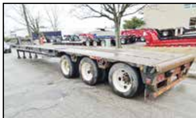
2008 XL SPECIALIZED XL100RG 50 TON, TRI AXLE, OILFIELD LOWBOY. AIR RIDE, FIXED NECK, 10" NECK, 40' DECK, 102" WIDE, CENTER ROLL, TAIL ROLL, 255/70 X 22.5 TIRES. CALL FOR MORE INFORMATION.
