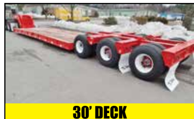
TALBERT 40 TON, 30' DECK, 18" DECK HEIGHT, 2 AXLE WITH PIN ON THIRD, AIR RIDE, HYDRAULIC DETACHABLE LOW BED. NON GROUND BEARING, DETACHES BOTH ENDS. SANDBLASTED AND PAINTED, NEW BRAKES AND SEALS, HUBCAPS, NEW DECKING, NEW DECALS & FLAPS, LO PRO TIRES, EX RIGGER TRAILER. LONG LOW LEVEL DECK. CALL FOR MORE INFORMATION.
