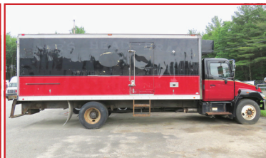
2008 HINO 338 28' Reefer Body. Diesel, Automatic, Air Brakes, PS, 200K Miles, $9,000.
