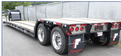
2019 FONTAINE RENEGADE LXL , 14" Deck Height, 30' Deck W/6" Ground Clearance, 2 Axle, Set Up For Third, Hydraulic Detachable, Taking Orders Call For More Information.
