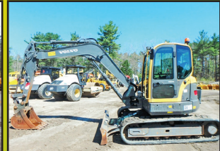
2013 VOLVO ECR88: 2,744 Hours, 22" Bucket, Cab, Auxiliary Hydraulics, 91" Blade, Swing Boom, Manual Coupler, 4 Cyl Volvo, 56 HP, 19K LB Size Class, stk#XC406, $49,500
