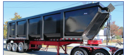
2019 KRUZ , 70 Yard, Tri Axle, 70,000 Single Point, Lift On Third Axle, 1/4 Inch 450 Hardox, Floor, Sides, Nose, Gate, 12 Panel Gate, 11 X 24.5 Rubber, Alum Wheels. Taking Orders. Call For More Information.
