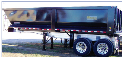
2019 KRUZ 26' STEEL TUB , Aluminum Frame Dump Trailer, Air Ride, 2 Axle, Alum Wheels, 450 Hardox, 24.5 16 Ply Tires. TAKING ORDERS Call For More Information.
