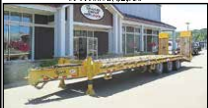
CAM SUPERLINE 25 TON DECKOVER. 8.5' x 30', 102" Wide, Air Ride, Tri Axle, Tool Box, #JP066336
