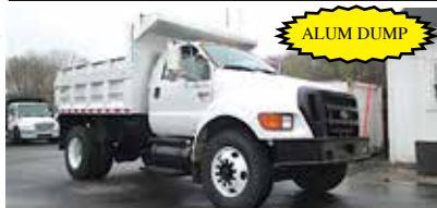
2005 FORD F-750 CAT C7 230HP., 72K ORIG. MILES, ALLISON 3000 RDS AUTO, 26K GVW, SPRING SUSP. W/ HELPERS, 11R 22.5 TIRES, DBL FRAME, AIR BRAKES, AIR SEAT, A/C, PTO, 10' ALUM. DUMP, 2 CHUTES, TARP, PINTLE REC. $36,500
