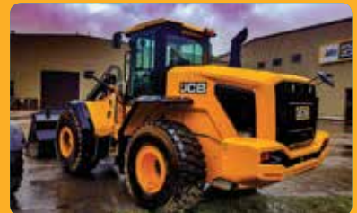
JCB 457HT #62593 46k lb, 4.6 cubic yd bucket cap, 256 HP, 23k load cap, 31' 1" dump clearance
