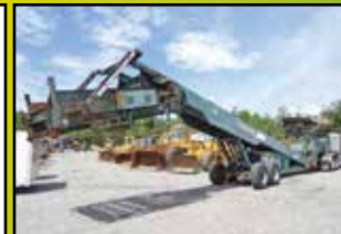
2000 POWERSCREEN COMMANDER 510: 3,545 HOURS, CONVEYOR STYLE SCREENING PLANT, 2" TOP SCREEN, 14" SLOTTED BOTTOM SCREEN, 4" GRIZZLY ON HOPPER, 4 CYL DEUTZ TURBO, 80 HP, VERY GOOD RUBBER, STK#SC361, $39,900
