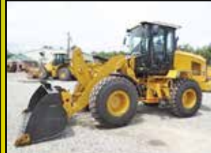
2014 CATERPILLAR 924K: 323 HOURS, 2.7 YARD, CAB W/ A/C, HYD COUPLER W/ 3RD VALVE, 6 CYL CAT TURBO, RIDE CONTROL, VERY GOOD RUBBER, 29K LB SIZE CLASS, STK#LO680, $125,500
