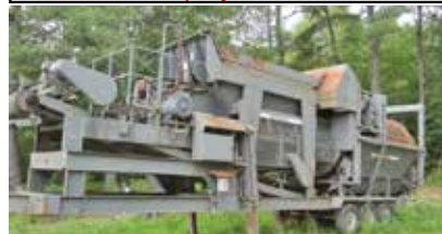
Rawson 613 Tromell Screen Plant. Deutz power, 6300 hrs, 50' stacker with Kubota diesel, mfg serviced, $59,500.
