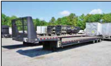
2000 LANDOLL TRI AXLE LOWBOY, 53' X 102", AIR RIDE, 10' NECK, HYDRAULIC SLIDING AXLE, BRADEN WINCH, 17.5 RUBBER. CALL FOR MORE INFORMATION.
