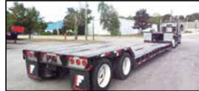
2014 FONTAINE LX40, NEW UNUSED, DOUBLE DROP TRAILER, 40 TON, MECHANICAL DETACHABLE, AIR RIDE, 2 AXLE, SET UP FOR THIRD, GOOSENECK EXTENSION CAPABILITY, 29' DECK, 9' 10" UPPER DECK, 9' 2" COVERED REAR BOGIE, 20" DECK HEIGHT, 255 RUBBER, D-RINGS, STAINLESS STEEL ACCENT PACKAGE. CALL FOR MORE INFORMATION.
