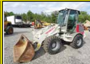
2012 TAKEUCHI TW65: 4,450 HOURS, 1.05 YARD, HYD COUPLER, CAB W/ A/C, 4 CYL DEUTZ TURBO, GOOD RUBBER, 11K LB SIZE CLASS, STK#LO923, $42,500
