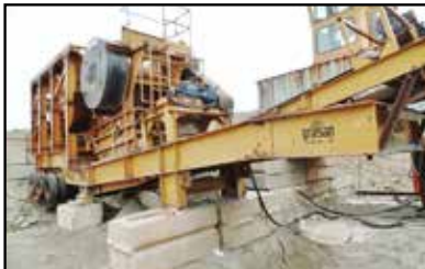
GRASAN 3042PE TRI AXLE PORTABLE JAW CRUSHER, HEWITT ROBBINS, 17' X 42" VIB FEEDER W/EXT. ELECTRIC DRIVEN, COMPLETE NEW BRAKE SYSTEM ON TRI AXLE CHASSIS, NEW ELECTRIC MOTOR, CONTROL PANEL AND CONTROL CABINET. WORKING DAILY. EXCELLENT SHAPE.
