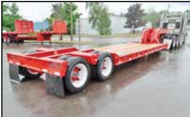
1994 ETNYRE 35 TON LOWBED TRAILER, NON GROUND BEARING, SPRING RIDE, 22' DECK, 102" WIDE, 2 AXLE, LO PRO TIRES, NEW 2" DECKING, SANDBLASTED AND PAINTED, NEW DECALS & DOT TAPE. EXCELLENT SHAPE. CALL FOR MORE INFORMATION.
