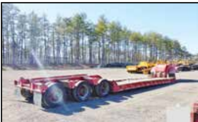
2005 TALBERT 55 TON TRI AXLE LOWBOY TRAILER, AIR RIDE SUSPENSION, HYDRAULIC DETACHABLE NECK, 25' DECK, 8' 6" WIDE, PLUMBED FOR BOOSTER, 255/70R X 22.5 RUBBER. CALL FOR MORE INFORMATION.
