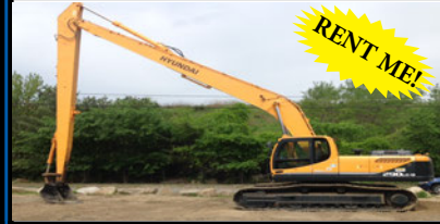
2011 HYUNDAI 290LC-9 CAB, A/C, 33'6" 65FT LONG REACH, 32" PADS, 36" DIGGING BUCKET. $145,000
