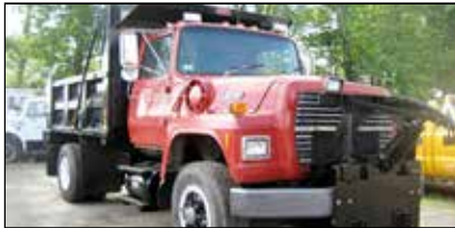
1990 FORD L8000 LOUIEVILLE. 210HP Ford diesel, 6 spd., air brakes, 36K GVW, 62K miles, 6 year Beau-Roc 8 yd. HD dump body, 1 chute, auto tarp, pintle hitch, central hyd., PA plow frame, sander controls, orig. paint & interior, new rubber, always garaged, needs nothing, 800-464-0573, www.WestsideTruckEquipment.com
