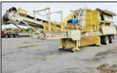
HEWITT ROBBINS 2540 PORTABLE JAW CRUSHER, 7' X 21' VGF FEEDER, 36" X 32' 6" FRONT DISCHARGE FOLDING CONVEYOR, TANDEM AXLE CHASSIS, HYDRAULIC LEVELING. CALL FOR MORE INFORMATION.
