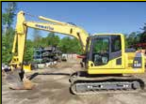
2012 KOMATSU PC130-8: 357 HOURS, 33" BUCKET, VERY GOOD U/C, A/C, 4 CYL KOMATSU TURBO, 8'6" WIDE, 2 SPEED, 28K LB SIZE CLASS, $97,500
