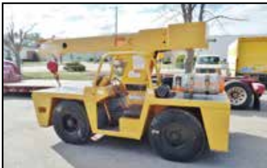
BRODERSON CARRY DECK CRANE, MODEL 1C801B, SERIAL # 108163, DECL LOAD CAPACITY 12,000 LBS, CENTERED ON AXLE, 17,000 LB MAX, BOOM EXTENDS 37'. CALL FOR MORE INFORMATION.
