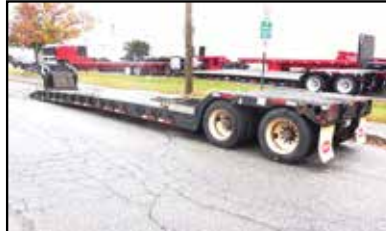
2008 FONTAINE 353, 35 TON TRAILER, 2 AXLE, SET UP FOR THIRD, NON GROUND BEARING, AIR RIDE, 30' DECK, 20" DECK HEIGHT, 102" WIDE, 255/70 X 22.5 RUBBER, OUTRIGGER BRACKETS, HONDA POWER PACK AVAILABLE, ONE OWNER, WORKING DAILY. CALL FOR MORE INFORMATION.
