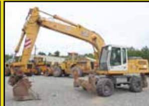
2000 LIEBHERR A914 LITRONIC: 42" BUCKET, CAB W/ A/C, WRIST & COUPLER, STABILIZERS, 4 CYL LIEBHERR TURBO, ALL-WHEEL DRIVE, 47K LB SIZE CLASS, STK#WX294, $27,500
