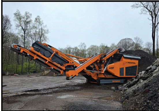
2025 ROCKSTER R1100DS BRAND NEW CLOSED CIRCUIT IMPACTOR. CAT ENGINE, CENTRAL GREASE SYSTEM, REMOTE CONTROL, MAGNET, SCREEN BOX, 2 WAY RETURN BELT. RENT OR PURCHASE! CALL FOR MORE INFO
