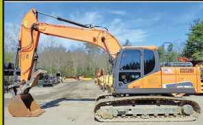
2021 DOOSAN DX180LC-5: 1,477 Hours, 44" Bkt, Hyd Doosan Thumb, 4 Cyl Perkins Turbo, Backup Camera, A/C, Good U/C, stk#XC692, $99,500
