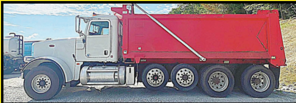
2015 PETERBILT 367 10X4, A/C, 485HP PACCAR MX-13 6CYL, ENG BRAKE, EF AUTO, STEERABLE AIR LIFT TAG AXLE, DBL FRM, HENDRICKSON HAULMAX, 18'L X 5'H HERITAGE STEEL BODY, ELEC ROLL TARP, HI-LIFT TAILGATE, 180K MI $99,000
