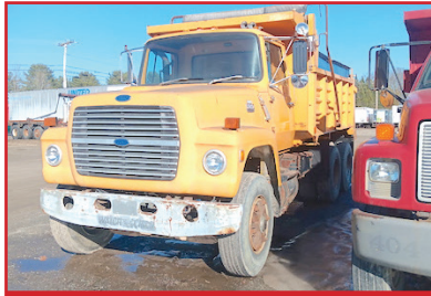
1985 FORD L8000 DUMP TRUCK. Tandem Axle, CAT 3208 Turbo, 8LL Trans., Hendrickson Suspension, $12,000
