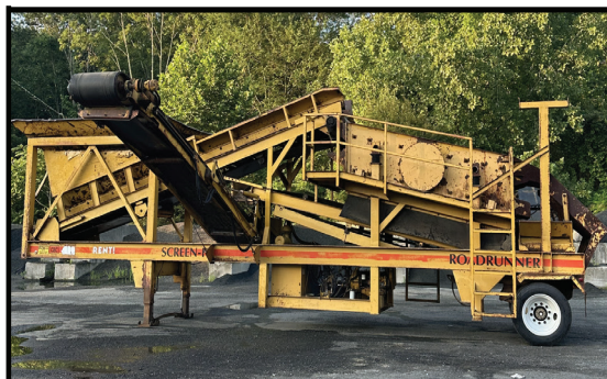
1999 CEC 4X10 3,345 HRS. RECENT OVERHAUL, ALL BRAND NEW HOSES, BELT, SCRAPERS. FULL SERVICE, NEW TIRES, BRAKES & LIGHTS ALL WORK. NEW SCREENS, BALL DECK. WORKING DAILY. $80,000
