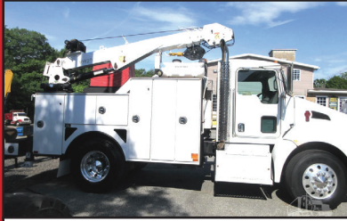
COMING SOON 2014 KENWORTH T370 SERVICE TRUCK. Paccar PX-9, Summit 10,000 lb Crane, Air Compressor, Lincoln Ranger 305G Welder/ 10500 Watt Generator, Power Inverter, Meter Reads 219,760 Miles, $91,900
