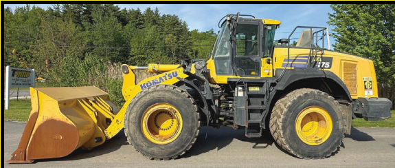
2022 KOMATSU WA475-10 A/C, AUX HYD, 128" JRB BKT, AUTOSHIFT, RIDE CTRL, REAR CAM, 775/66R29 RADIALS, 10,918 HRS
