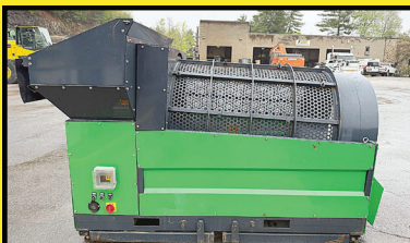
EINGP GF480 20-40 TON/HR ROTARY DRUM TROMMEL SCREEN, 4'8"X2'11" TROMMEL, 2'2"X4'10" FDR HPR 3-PHASE ELEC MOTOR, FORKS POCKETS $4,500
