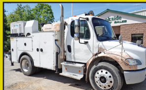
2016 FREIGHTLINER BUSINESS CLASS M2: 267,342 Miles, Cummins ISB6.7, 240 HP, Allison RDS 2500 Auto, 25.5k GVW, IMT 8600-22 Crane, stk#TK761, $39,500
