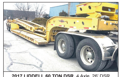
2017 LIDDELL 60 TON DSR. 4 Axle, 26' DSR Deck, 9' Wide, 8'6" Bogie, 26' Beam Deck, 4th Axle, Alum Wheels, Gooseneck Extension, Power Pack, Excellent Shape, Call For More Information.
