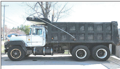
1999 MACK RD688SX DUMP TRUCK. 350 Mack Motor, 8 Speed, 58K Rears, 24" Rubber, 15.6 Body, Pintle Hook, Scuttle Doors, P/S, Jake Brake, A/C, 256K Original Hours. Call For More Information.
