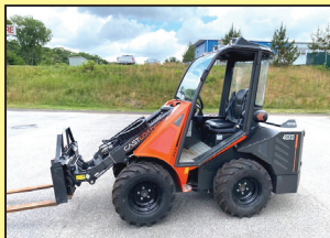
CAST 40XD LOADER. 40 HP, 3000lb Capacity, Aux Hydraulics, Telescopic Boom
