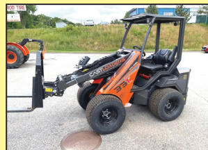
CAST 33TLC CARBON. 23 HP, 2200lb Capacity, 2 Speed, Aux Hydraulics, Telescopic Boom
