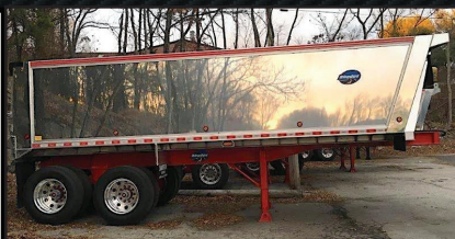
2023 RHODES ASS2660-2 26' ALUM. DUMP TRAILER , Steel Frame, Single Point Suspension. Incoming! 401-434-5900
