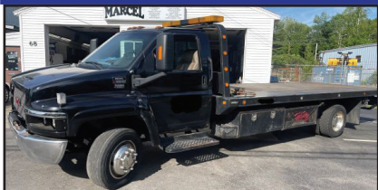
2006 GMC C5500 ROLLBACK TRUCK, New Injector, New Turbo, New Alternator, Tires 6 Months Old, Rubber 80%, Transmission Good, Good Shape & Ready To Work. $24,900 Call Today! 781-417-3018
