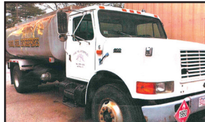
1997 IH 4900 3000 GALLON TANK. Boston Reel, Bottom Load, DT-466, 6 Speed, 33,000 GVW, Steel Tank, $6,900
