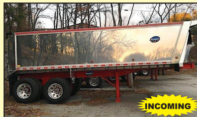
2023 RHODES ASSS2660-2 26' ALUMINUM END DUMP TRAILER, STEEL FRAME, SINGLE POINT SUSPENSION. INCOMING !
