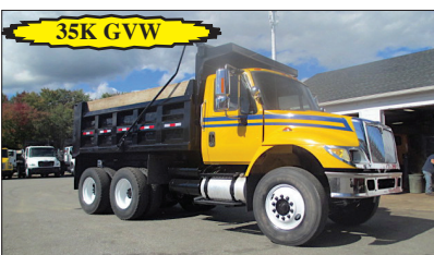
35K GVW 2003 INTERNATIONAL 7400: DT530-285HP, 8LL, 54K GVW, SPRING SUSP., EXHAUST BRAKE, EXHAUST BRAKE, 11R 22.5 TIRES, DBL FRAME, AIR-BRAKES, A/C, PTO, 14" STEEL DUMP, ELECTRIC TARP, AIR-GATE, PINTLE PLATE. $43,000
