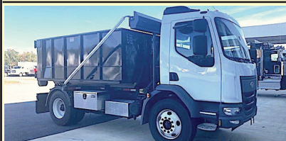
2022 PETERBILT 220 : UNDER CDL, PACCAR PX-7 260HP, ALLISON 2500RDS TRANS., AMERICAN HOOK-LIFT, HAD-185- 120-36/54 HOIST WITH AN ADJUSTABLE JIB FROM 36"-54" AND CAPACITY OF 20,000#. HANDLES CONTAINERS FROM 10-14 FEET.
