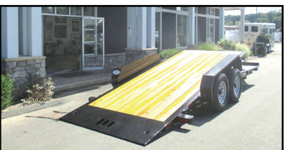
CAM SUPERLINE 15.4K EXTRA WIDE SPLIT TILT TRAILER. 6' 11" x 21', Slipper Spring Suspension, #527506
