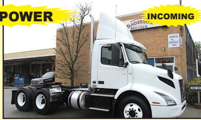
2023 VOLVO VNR64T300-D13, 435HP, I-SHIFT AUTOMATIC, 12,000# FRONT AXLE / 40,000# REAR AXLE, REGIONAL DISTRIBUTION.
