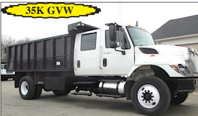
35K GVW 2013 INTERNATIONAL 7400: DT466-260HP, 69K MILES, ALLISON 3500RDS AUTO, SPRING SUSP., LOCK DIFF., SINGLE FRAME, 11R 22.5 TIRES, AIR-BRAKES/SEAT, PTO, NEW 15" STEEL DUMP, 4" SIDES, BARN DOORS, PINTLE HITCH, AIR-TO-REAR. $49,000
