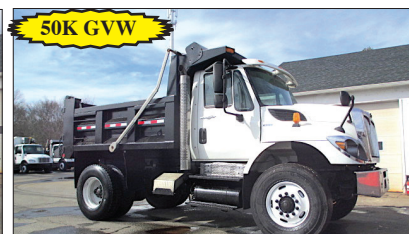
50K GVW 2010 INTERNATIONAL 7400: DT530-300HP, 119K MILES, EXHAUST BRAKE, ALLISON 4500RDS AUTO, 50K GVW, SPRING SUSP., 7.16 GEARED RATIO, DBL FRAME, 315/80R 22.5 TIRES, AIR- BRAKES/SEAT, PTO, 10" STEEL DUMP, AIR-GATE, ELECTRIC TARP, PINTLE HITCH. $59,000
