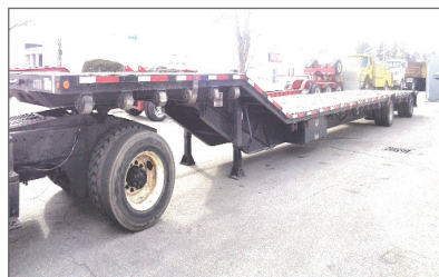
2011 DOONAN 53' SPREAD AXLE STEP DECK, 8'6" Wide, 120 Inch Axle Spread, Air Ride, 10' Top Deck, 38' 6" Lower Deck. Call For More Information.
