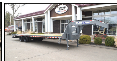
SURE-TRAC 22.5K LOW PROFILE DECKOVER GOOSENECK. 8' 6" x 30', 25' Deck + 5' Beavertail, Bi-Directional Springs In Ramps, #331439
