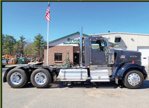
2004 KENWORTH W900: 467,030 Miles, 10 Wheel Day Cab, Cat C15, 475 HP, Fuller 18 Speed, Air Ride, 13.2K F, 46K R, Wetline, stk#TK859, $67,500
