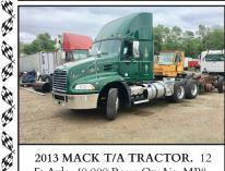
2013 MACK T/A TRACTOR. 12 Ft Axle, 40,000 Rears On Air, MP8, 10 Speed Fuller, Very Clean, Fleet Maintained, 630K Miles, \$32,500
