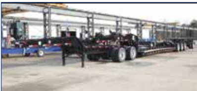
2019 FONTAINE 60 TON MODULAR 2+3+1 , 26' Dsr, 184" Swing Clearance, Set Up For 2 Axle Jeep, 14" Deck Height, Air Ride, Alum Wheels, 275/70R X 22.5 Rubber, Non Ground Bearing. Call For More Information.
