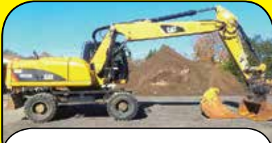
2010 CAT M322D CAB, A/C, FRONT BLADE, VA BOOM, 8'2" STICK, AUX HYD, Q/C, 36" BKT, 8000+/- HRS, 60" TILT AVAIL $129,500
