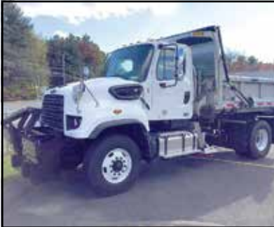
2017 FREIGHTLINER 114SD PLOW TRUCK. Detroit DD13, 370 HP, 10' Monroe 5-7 Yard Body, Monroe Snow Plow, Power Cover, PS, PW, PL, Stk# JB2422
