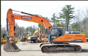
2020 Doosan DX350LC-5: 3,394 Hours, 61" Strickland Bucket, Very Good U/C, 6 Cyl Doosan, A/C, 78K Lbs, stk#XC510, $94,500
